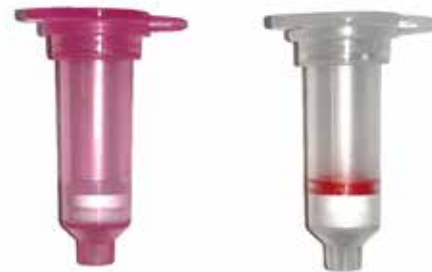
Figure 3. Comparison of PureLink and Qiagen columns. The PureLink column (right) has a larger bed than the Qiagen column (left), supporting higher input capacity.
