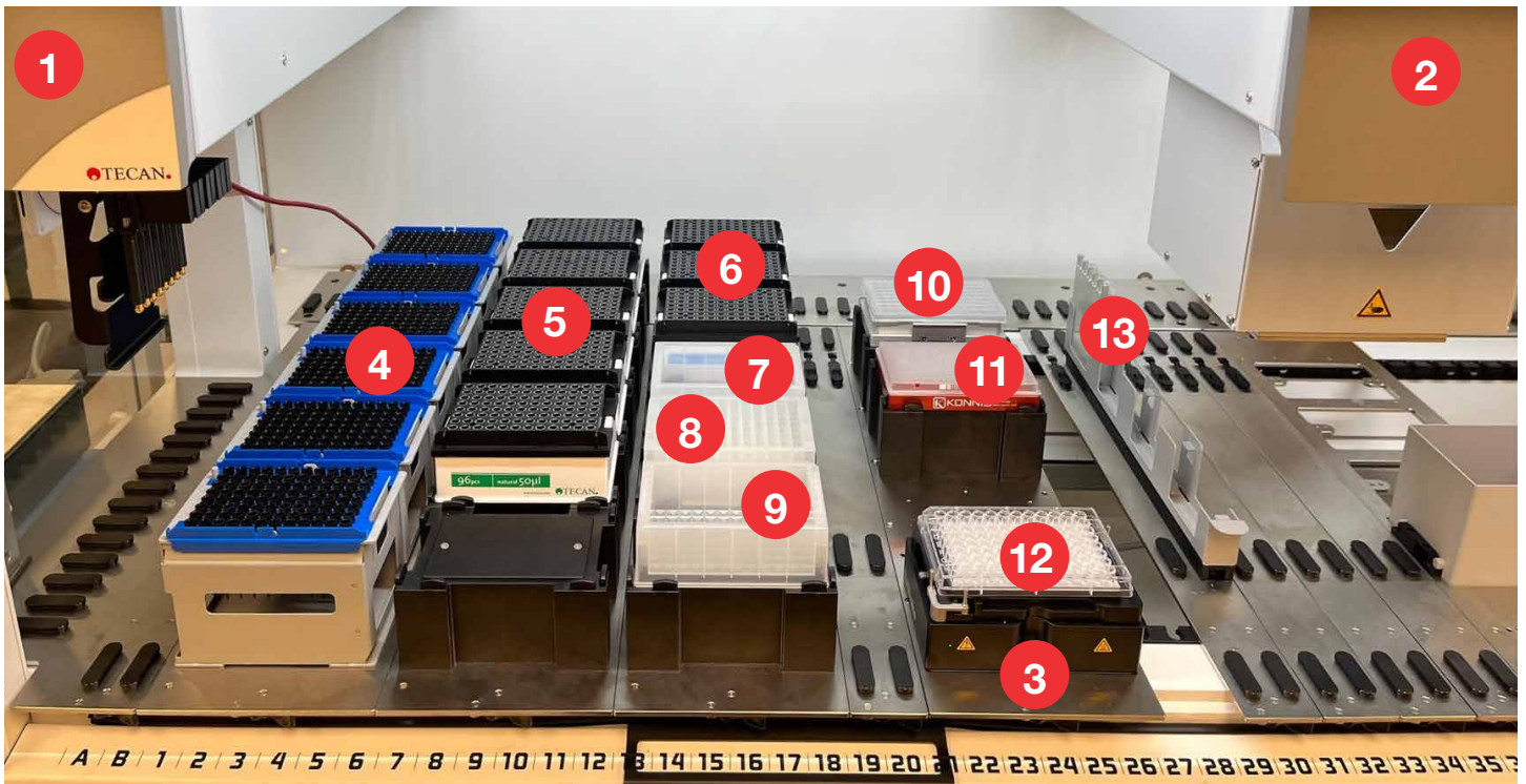
Figure 2. Configuration deck of the Fluent 780 system as outlined and described in Table 1 below.
