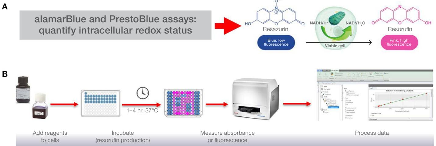
**Figure 2. Resazurin-based alamarBlue and PrestoBlue assays. (A)** Schematic example of intracellular reduction of resazurin by NADH-dependent enzymes. **(B)** General protocol used for measurement of alamarBlue and PrestoBlue assays using the Varioskan LUX multimode reader.
