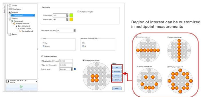
**Figure 3. SkanIt Software 5.0 protocol for detection of resorufin fluorescence intensity in alamarBlue and PrestoBlue assays.**
