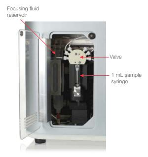
Figure 31. Positive-displacement syringe pump. The syringe is easily removed for cleaning or replacement.
