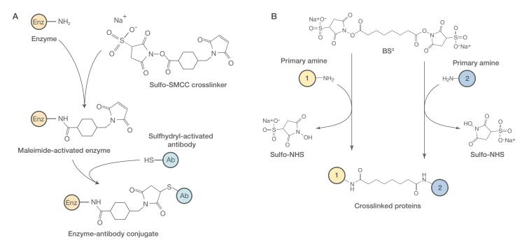
Figure 12. Example reactions for producing detection conjugates. (A) Enzyme–antibody conjugation with heterobifunctional crosslinker Sulfo-SMCC. (B) Use of homobifunctional crosslinker BS<sup>3</sup>.
