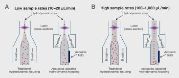
Figure 27. Acoustic focusing vs. traditional hydrodynamic focusing as particles pass through the laser. (A) In acoustic focusing, cells remain in tight alignment even at higher sample rates, resulting in less signal variation and improved data quality. (B) In traditional hydrodynamic focusing, increasing the sample rate results in widening of the sample core stream, resulting in increased signal variation and compromised data quality.
