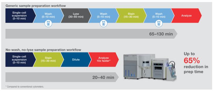
Figure 32. No-wash, no-lyse sample preparation workflow.
