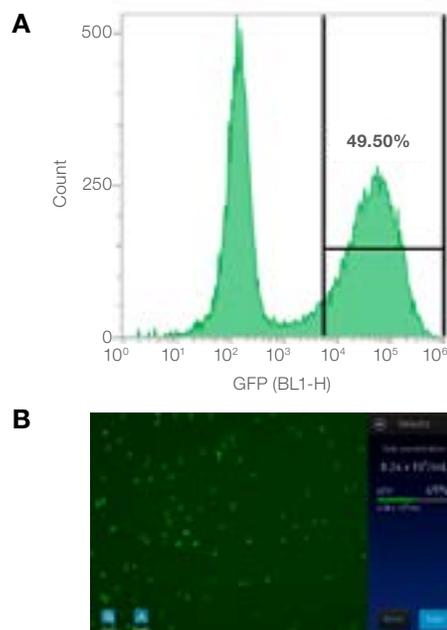
**Figure 4. Fluorescent cell counts similar to those obtained by flow cytometry can be easily acquired with the Countess II FL Automated Cell Counter, with a single light cube.** U2OS cells were transduced using Invitrogen™ CellLight™ Nucleus-GFP, BacMam 2.0, and allowed to incubate for 36 hours. The cells were evaluated for GFP on (A) a flow cytometer and (B) the Countess II FL Automated Cell Counter. The proportions of transduced cells determined by the two methods are nearly identical.
