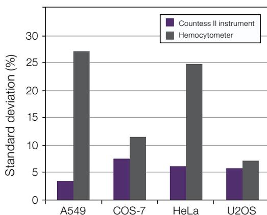
**Figure 5. User variability when counting with a hemocytometer compared to using a Countess II instrument.** Identical samples of A549, COS-7, HeLa, and U2OS cells were counted by three different operators using a Countess II instrument and then manually with a hemocytometer and microscope. The user-to-user variability is much higher for the hemocytometer than for the Countess II instrument.
