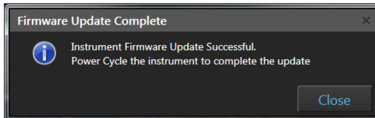
**Step 5** **Power Cycle** the instrument (turn off, then on) to complete the firmware update.
