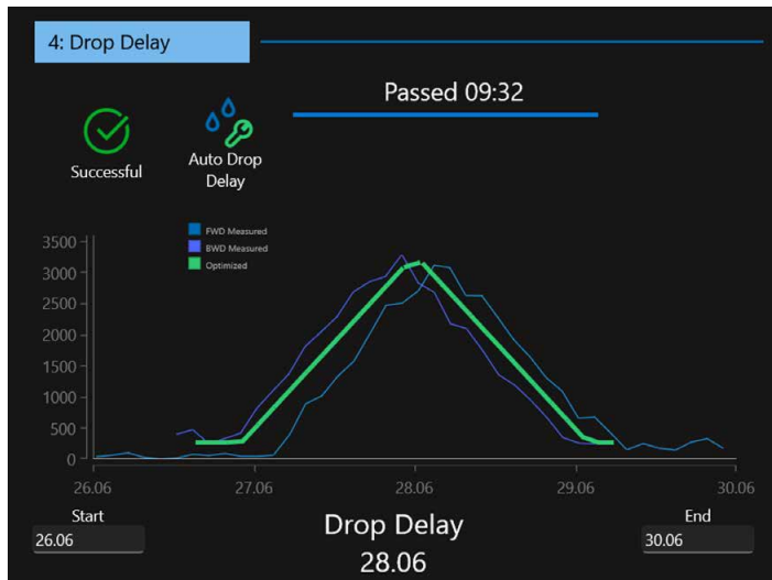
Figure 5. A representative screenshot of the automated drop delay plot. The Bigfoot Cell Sorter uses fluorescent beads and a miniature cytometer to advance through increasing and then decreasing increments of drop delay settings. The initial starting point for these scans is based on historical reference settings for the nozzle size and instrument serial number. The mean drop delay of the maximum signals detected in each direction is selected as the optimized drop delay setting.
