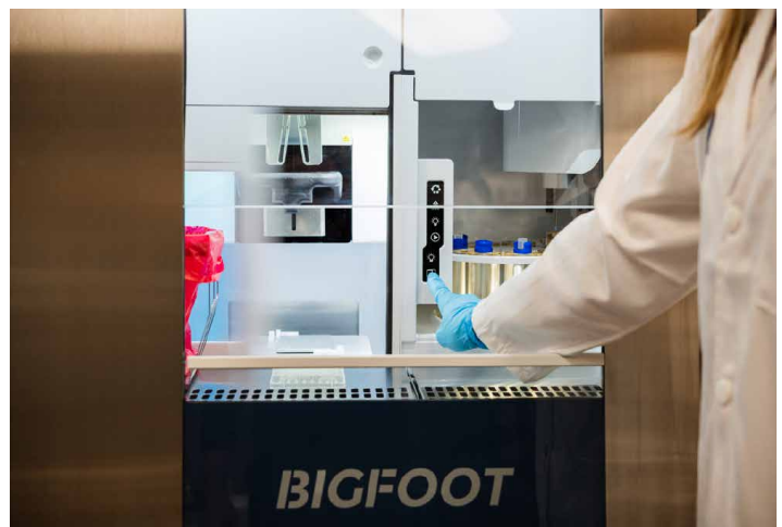
Figure 4. The internal control panel limits the need for the operator to reach in and out of the BSC.
