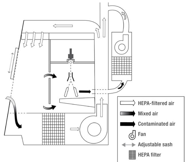
Figure 1. Airflow diagram.
