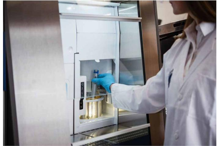
Figure 2. Adjustable sash in the up position for sample access.
