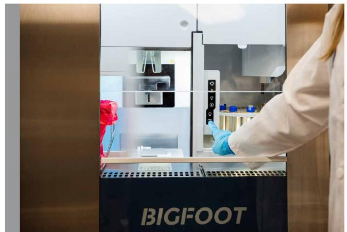
Figure 4. The internal control panel that limits the need for the operator to reach in and out of the enclosure.
