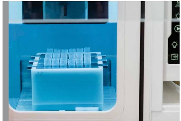
Figure 3. The sort collector with numerous sort tubes.
