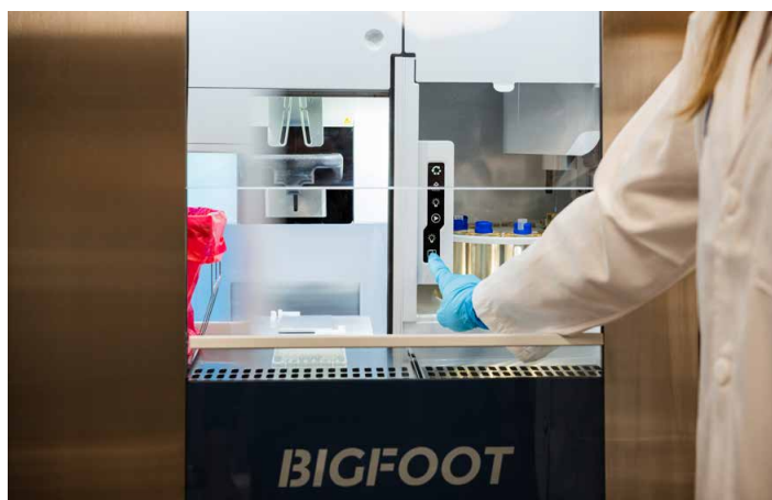
Figure 3. The multi-sample loader is inside the BSC.
