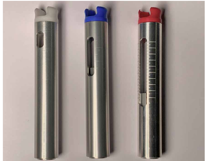
Figure 2. Sample input tube adapters for 1.5 mL (white), 5 mL (blue), and 15 mL (red) tubes.
