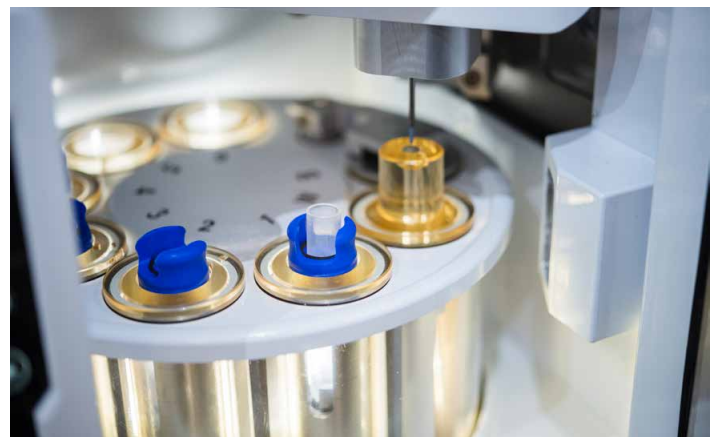
Figure 1. The multi-sample loader on the Bigfoot Spectral Cell Sorter is shown with the sample probe above the wash station.
