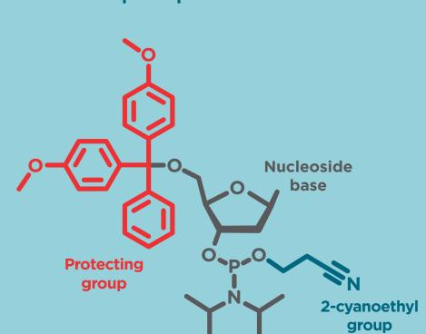
chemical building blocks of oligo synthesis, consist of a protecting group (e.g., dimethoxytrityl, DMT) and a cyanoethyl reactive group.
