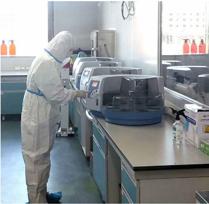
Nucleic acid extraction from patient samples with the KingFisher Flex Purification System.
