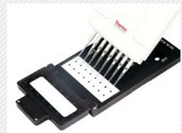
Samples are easy to pipette onto the plate with a single- or an eight-channel pipette.
