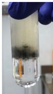
Sucrose cushion: 50% sucrose in TNE buffer (20 mM Tris- HCL (pH 7.0), 100 mM NaCl, 2 mM EDTA)
