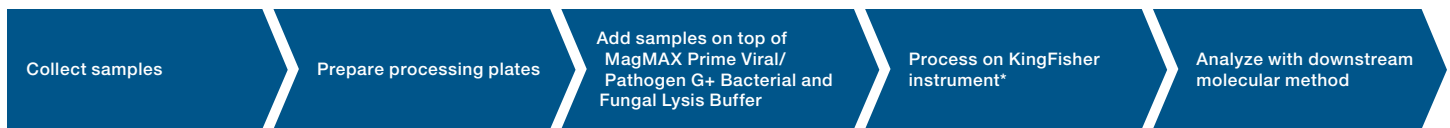
Figure 2. Advanced lysis workflow of the MagMAX Prime Viral/Pathogen kit for difficult-to-lyse gram-positive bacterial and fungal targets.
