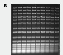
Gel stained with SYBR Gold dye and imaged on an iBright Imaging System
