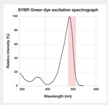
Figure 23. The iBright green LED transilluminator effectively excites common DNA stains. Excitation spectrographs of (A) ethidium bromide, (B) SYBR Gold dye, and (C) SYBR Green dye (purple lines). The 490–520 nm emission range of the iBright transilluminator is indicated by the light red boxes.
