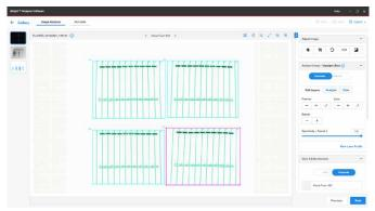
Figure 17. Analysis workspace in iBright Analysis Software. Four separate blots were analyzed using the automatic analysis feature. The blots were identified in four independent analysis frames that could be edited and analyzed separately.
