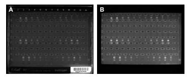
Figure 10. Imaging with iBright Tray Adapters helps prevent fluorescence emitted by the E-Gel cassette barcode and label from interfering with the algorithm used by Smart Exposure technology. Images of an E-Gel 96-well agarose gel captured (A) without and (B) with an iBright Tray Adapter.
