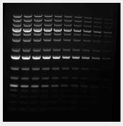
Gel stained with ethidium bromide and imaged using a UV transilluminator-based imaging system
