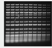
Gel stained with SYBR Green dye and imaged on an iBright Imaging System
