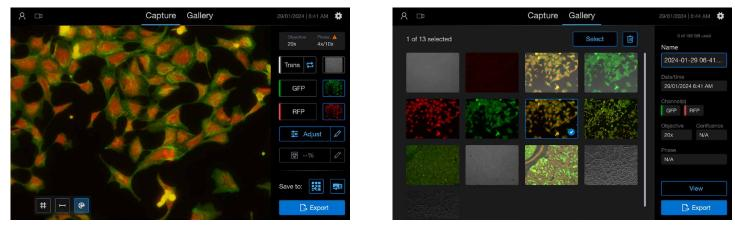
Figure 8. Powerful onboard software with image processing tools built in. The easy-to-use EVOS M3000 Imaging System UI enables you to easily capture images in transmitted light or fluorescence (left) and explore saved images with the image gallery (right).
