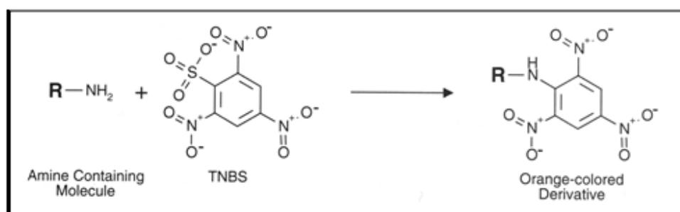
Reaction of TNBSA with a primary amine-containing molecule to produce a chromogenic derivative.
