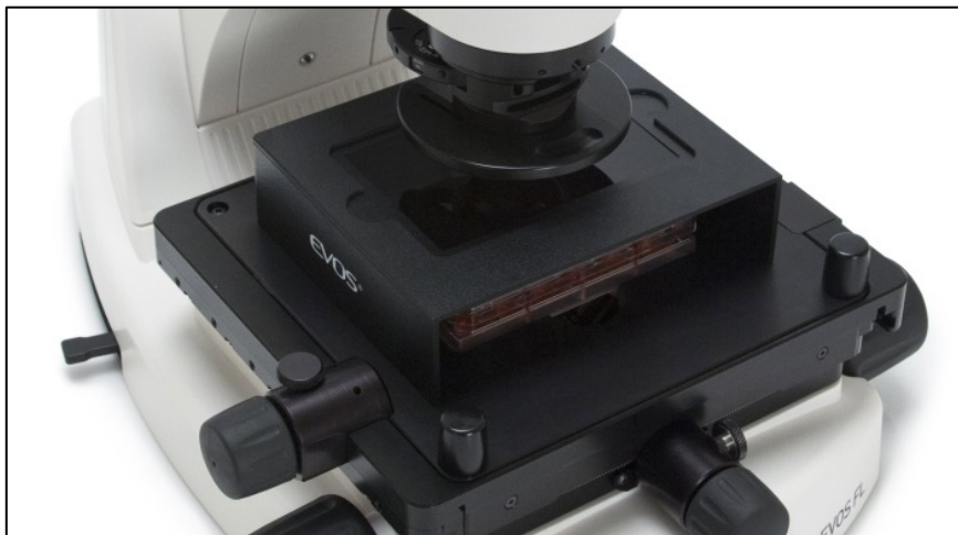
Light shield box on stage
