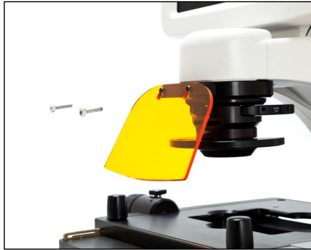
Secure the UV shield in place
