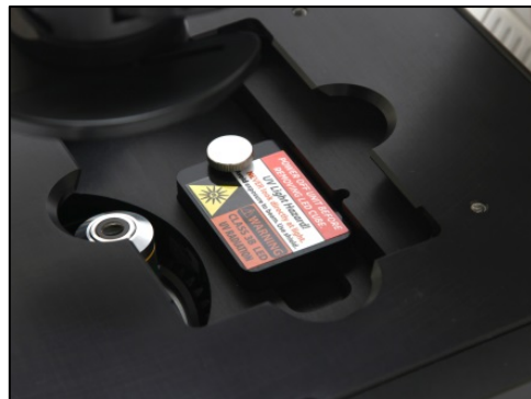
Light cube access cover (under stage)
