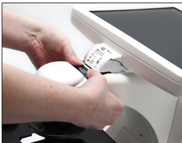
Grasp under support arm with both hands to lift the instrument
