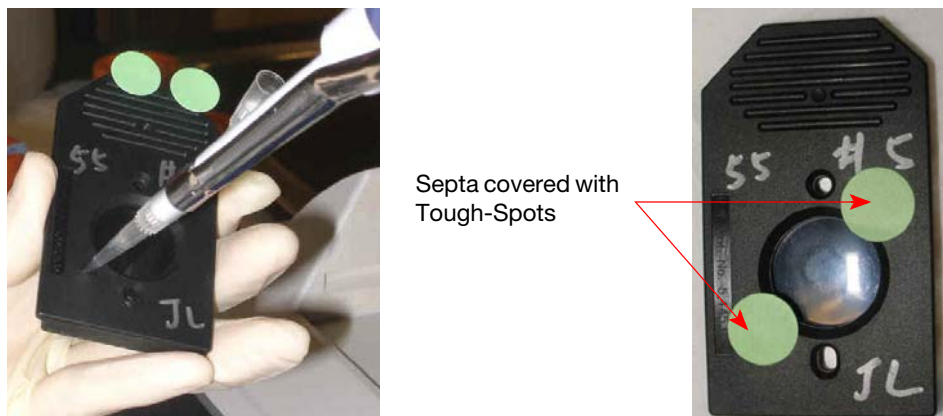
Figure 20 Loading samples onto arrays
