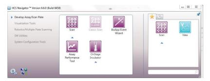
If the Onstage Incubator button does not appear, Click **System Configuration Tools**, double click the **ArrayScan Config** button, Click **On Stage Incubator**, Click the box next to **Enable On Stage Incubator**, Save the configuration and close the window. See the figure below.
