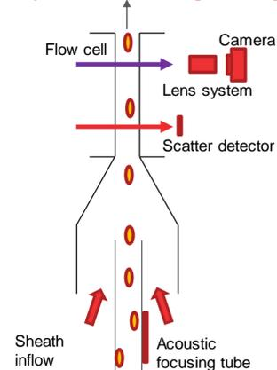
The sample flows up through an acoustically driven tube where particles are aligned along the axis. The sample stream is then injected into a sheath stream. Particles travel up through a scatter detector system that sends a delayed trigger to the camera.
