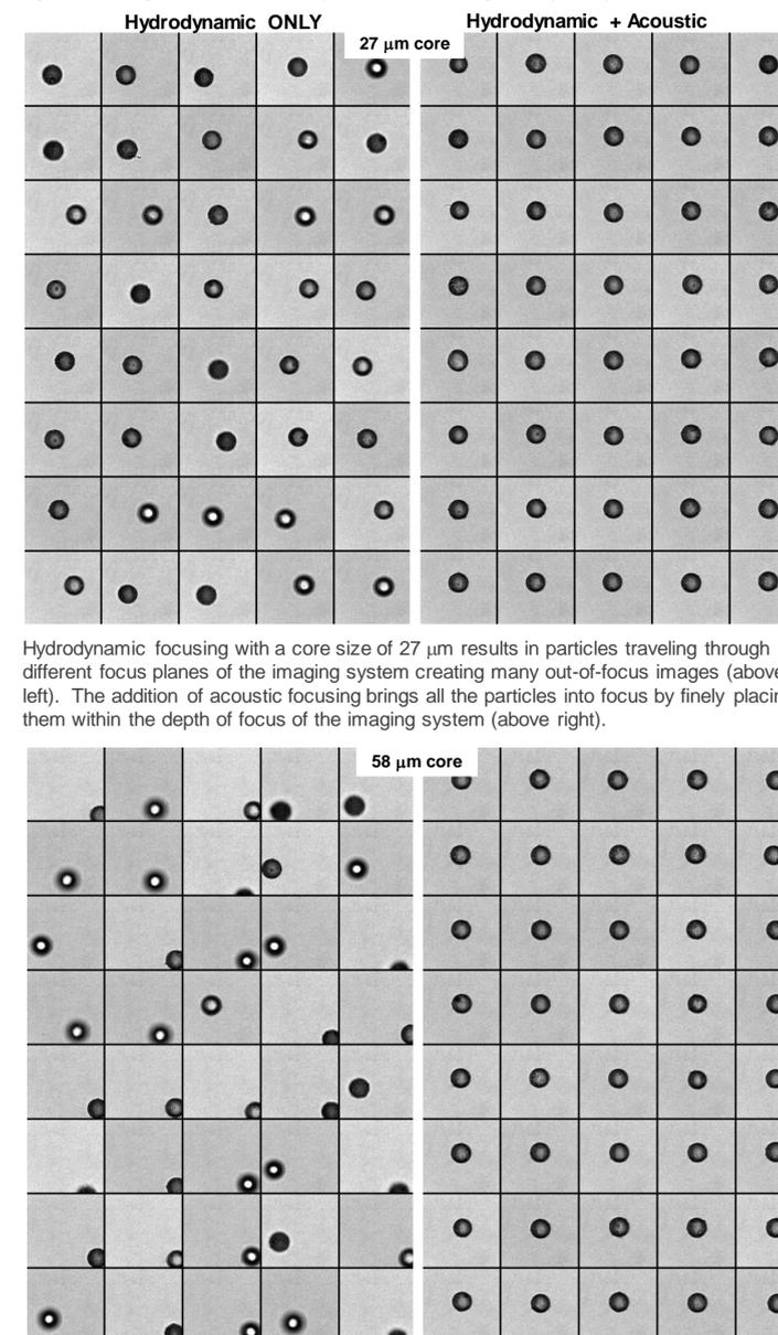
Hydrodynamic focusing with a core size of 27  $\mu\text{m}$  results in particles traveling through different focus planes of the imaging system creating many out-of-focus images (above left). The addition of acoustic focusing brings all the particles into focus by finely placing them within the depth of focus of the imaging system (above right).
