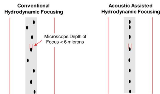
Particles in a hydrodynamically focused flow system (left) are distributed throughout the core stream. For most flow cytometers the core diameter is larger than the depth of focus. Acoustic focusing (right) is used to further align the particles within the core stream to contain them within the depth of focus.
