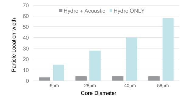
Range of particle locations for different core stream diameters. For hydrodynamic focusing only, in most cases, the particles are distributed across the core and their spread is thus approximately equal to the core size. Adding acoustic focusing limits the particle spread to < 5 microns.
