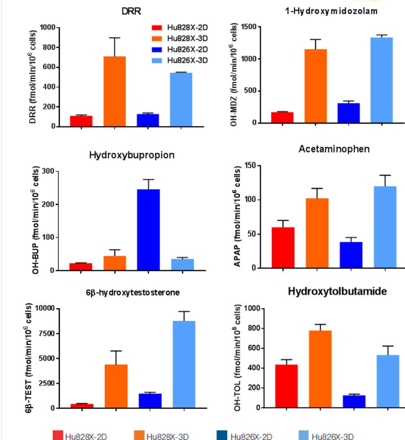
The metabolites quantified using HRMS were converted to mole amounts based on the standard curves of the respective metabolites. Two different lots of PHH, Hu828X and Hu826X (partially redacted), were used in this assay. Results were normalized to incubation time of individual substrates and number of cells per well in the 2D and 3D cultures. Data is the mean  $\pm$ SD; n = 3.
