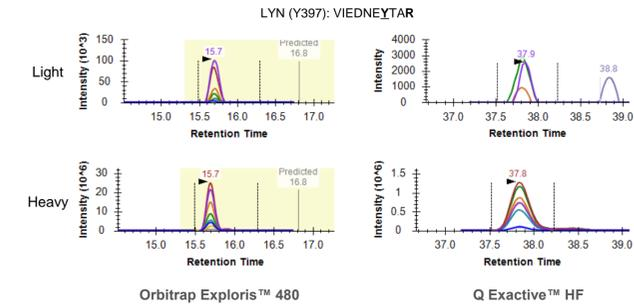
PRM analysis of SMOAC enriched phosphopeptides from A549 (+hIGF) and HeLa (+hEGF) resulted in accurate and precise quantitation of 134 heavy IS phosphopeptides. Improved signal to noise and sensitivity was observed with new Orbitrap Exploris™ 480 (Figure 6). Differential expression of many phosphopeptides observed between two cancer cell lines (data not shown).
