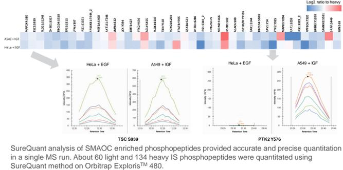
SureQuant analysis of SMAOC enriched phosphopeptides provided accurate and precise quantitation in a single MS run. About 60 light and 134 heavy IS phosphopeptides were quantitated using SureQuant method on Orbitrap Exploris™ 480.
