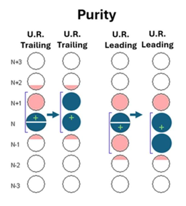
Figure 1: For purity and enrich modes, the ultra-recovery option can be enabled. If the positive particle is in the leading or trailing ½ of the droplet (blue), and there are no particles in the adjacent (red), an additional drop will be sorted to increase the recovery of the positive particles. Note that for purity mode, the adjacent area extends ¼ drop farther to ensure that the purity isn't compromised, while in enrich is uses a smaller scatter adjacent area to maximize recovery.
