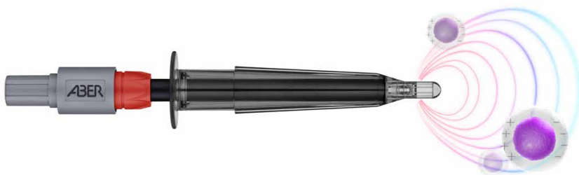
Figure 1. Aber Futura Neo biocapacitance sensor, and representation of measurement field.
