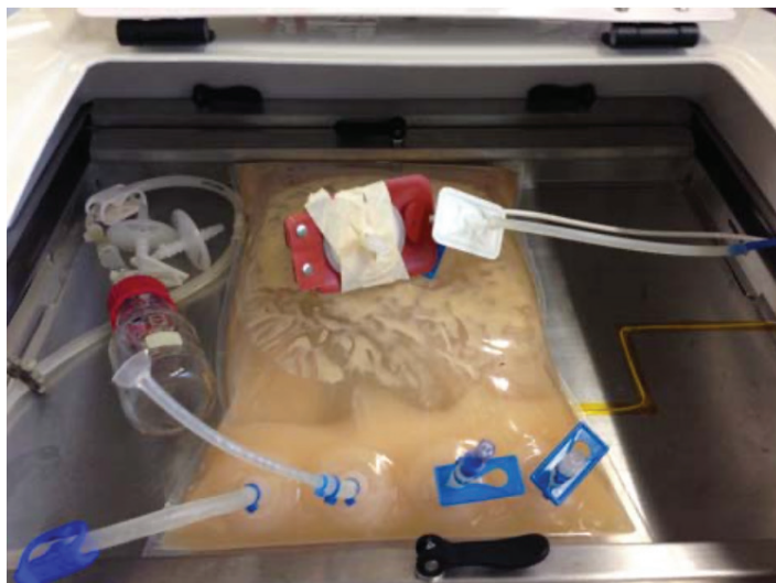
Figure 2. The BY-2 tobacco cell culture in the HyPerforma Rocker Bioreactor BPC after seven days of culture. The specially designed sampling system is shown on the left side.
