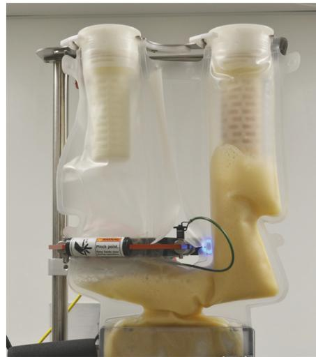
Figure 2. Pinch clamp preventing fouling of the back-up exhaust filter in case of accidental foam-out. The exhaust filter shown was intentionally foamed out to validate the effectiveness of the pinch clamp.
