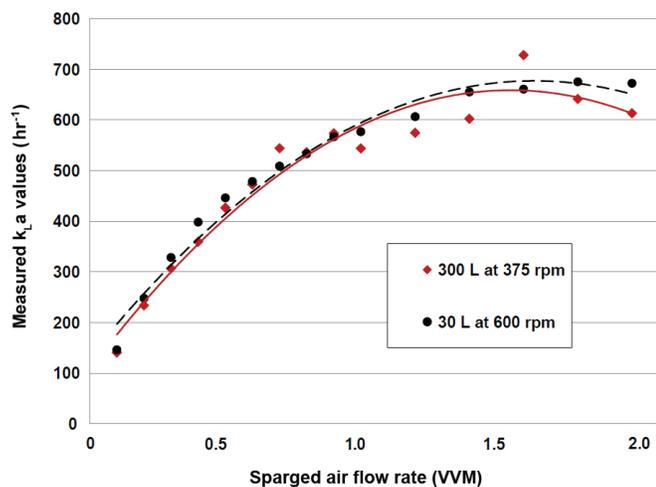
Figure 3. Oxygen delivery in the 30 L and 300 L S.U.F.s was about  $650 \pm 25 \text{ hr}^{-1}$  at maximum agitation rpm and air flow rates of 2 VVM in 10 g/L NaCl in DI  $H_2O$  test solution.
