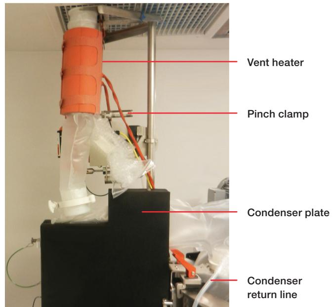
Figure 1. Exhaust filters, pinch clamp, and condenser on the 300 L S.U.F.
