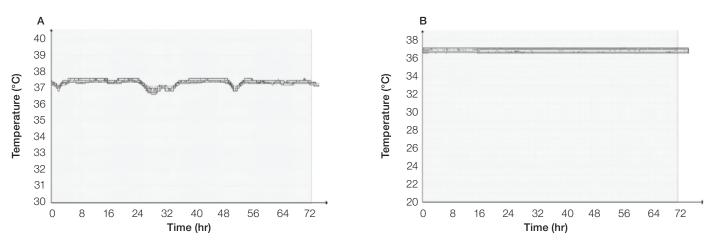
Figure 5. Temperature curve of (A) ordinary incubator and (B) Nunc Cell Factory incubator.
