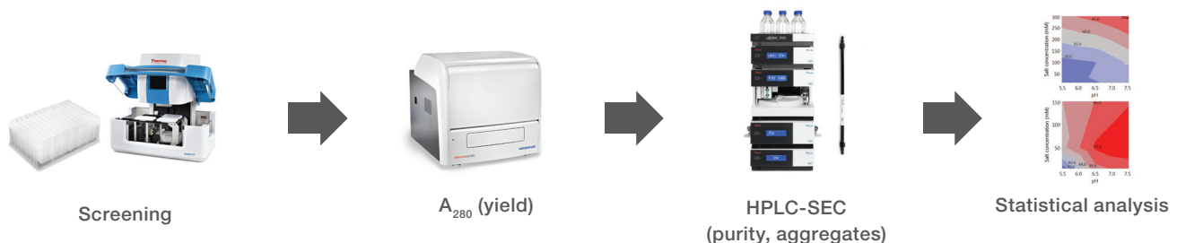
Figure 3. The general workflow for aggregate removal consists of filter-plate screening followed by A_{280} concentration determination and purity analysis by HPLC-SEC; statistical analysis is used to generate trends and to select process conditions.
