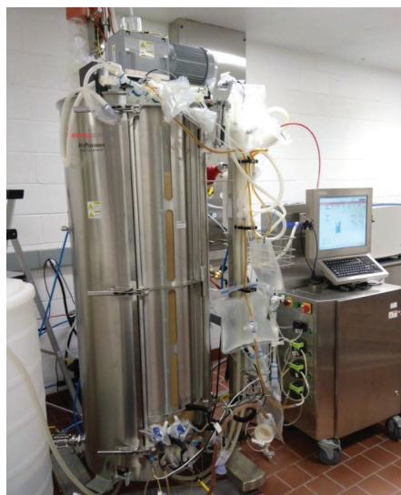
Figure 1. 300 L HyPerforma S.U.F. with Thermo Scientific™ HyPerforma™ G3Lite™ controller and Prima BT off-gas analyzer.
