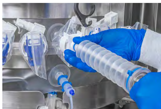
Figure 3.81. Installing the pre-sterilized sensor.
