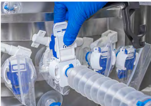
Figure 3.78. Squeezing connectors together.
