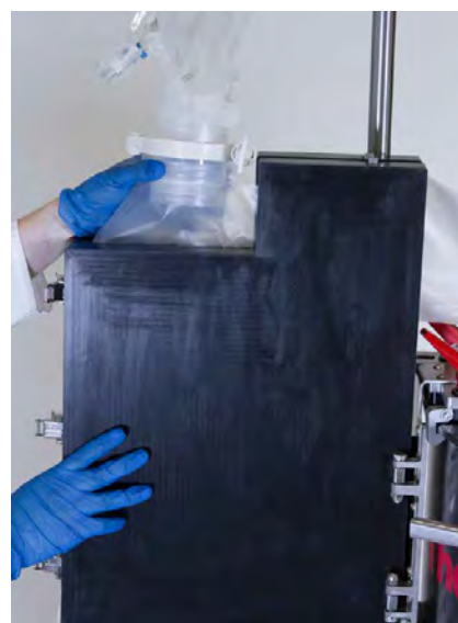
Figure 3.40. Closing the condenser door.
