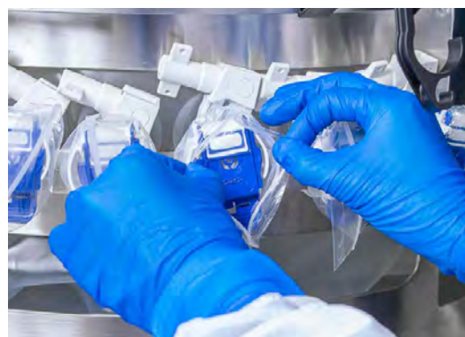
Figure 3.75. Removing the plastic covering from the connector.
