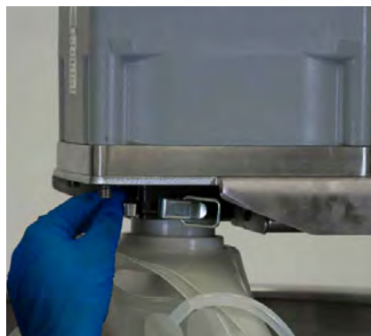
Figure 3.38. Latching the bearing port.
