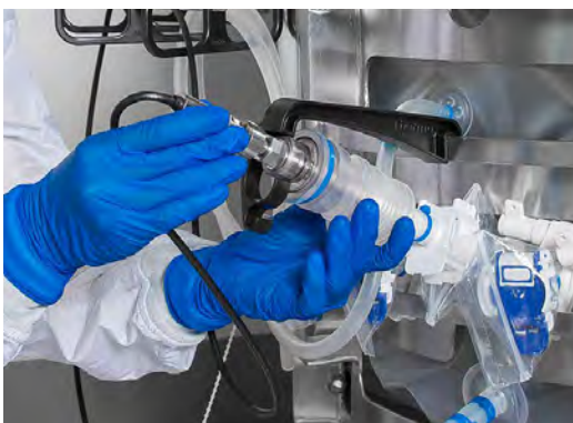
Figure 3.83. Lifting the probe upward into the spring.
