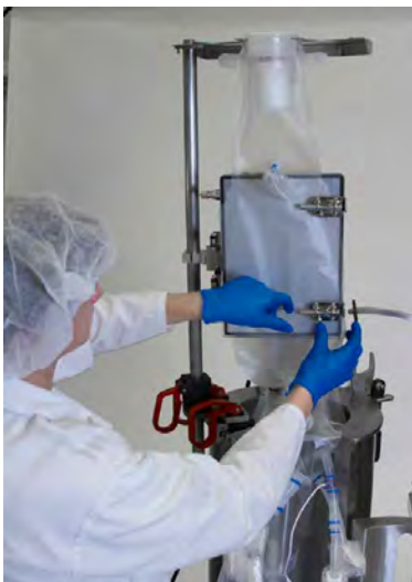
Figure 3.7. Loading of an optional condenser bag.
