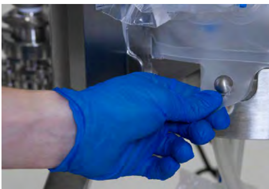
Figure 3.12. Aligning a hanging tab with the pin.
