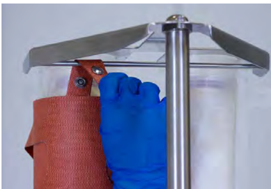
Figure 3.8. Installing an exhaust filter heater.
