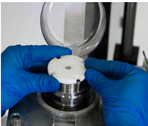
Figure 3.55. Aligning the motor drive keyway with the drive shaft head slots.
