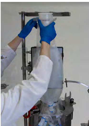
Figure 3.6. Inserting a vent filter into the filter bracket.
