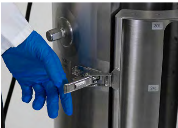
Figure 3.1. Opening the S.U.F. door latch.
