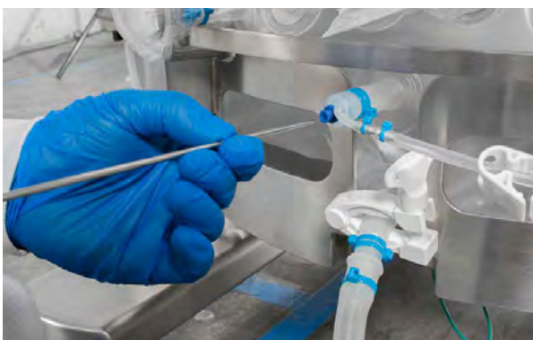
Figure 3.61. Inserting a sensor into the thermowell.
