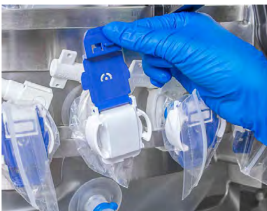
Figure 3.76. Opening the protective cover pull tab on the port.
