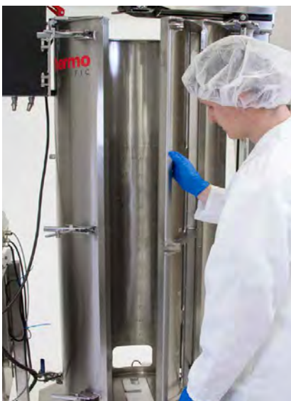
Figure 3.30. Opening the fermentor door.
