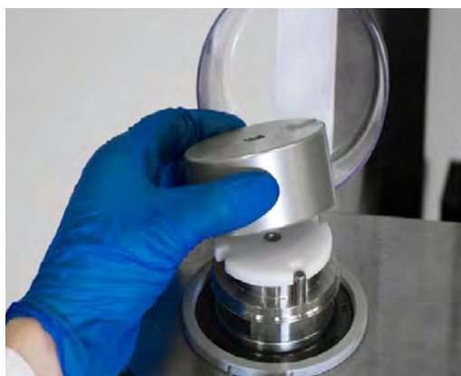
Figure 3.56. Replacing the drive shaft cap.
