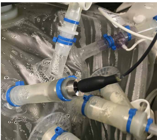
Figure 3.62. Foam sensor wire connected in port.
