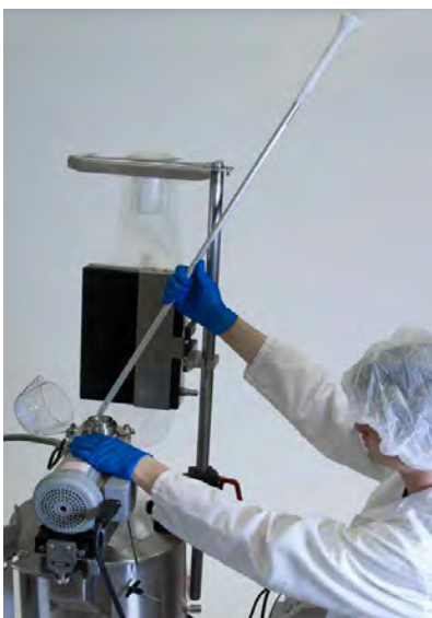
Figure 3.20. Using two hands to load the drive shaft.
