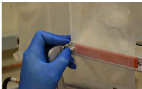
Figure 3.15. Positioning the BPC cutout over the alignment pin in a pinch clamp.
