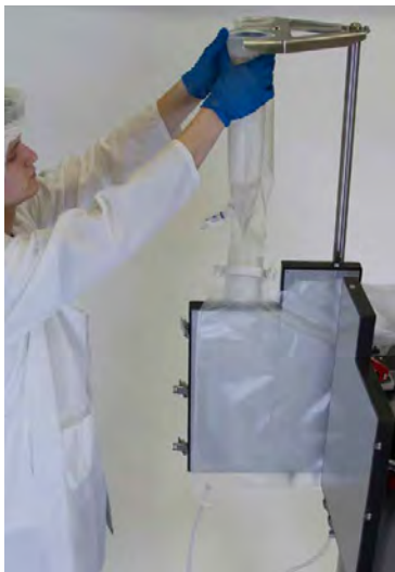
Figure 3.66. Positioning the condenser BPC and vent filter in bracket.
