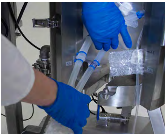
Figure 3.5. Routing the sparge and bottom drain lines.
