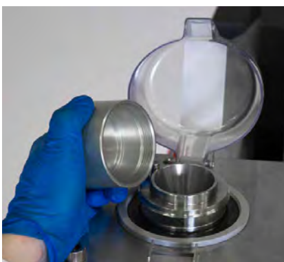
Figure 3.50. Removing the drive shaft cap.
