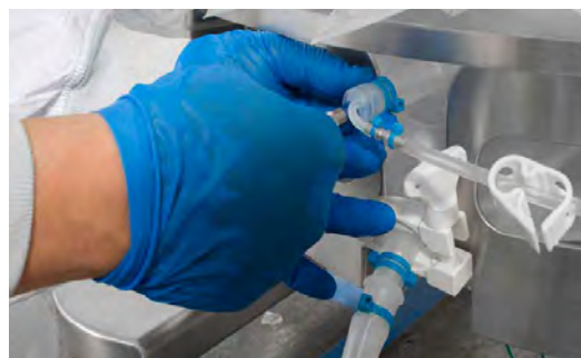
Figure 3.27. Securing the RTD by twisting the luer lock collar.
