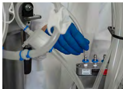
Figure 3.11. Incoming line connection to a direct sparger filter.
