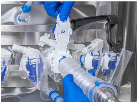
Figure 3.79. Pulling tabs to remove the paper membranes.
