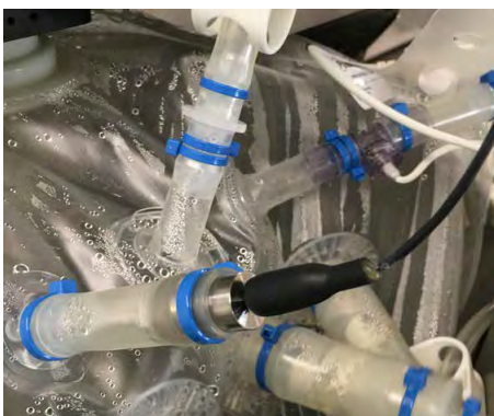
Figure 3.28. Foam sensor wire plugged in.
