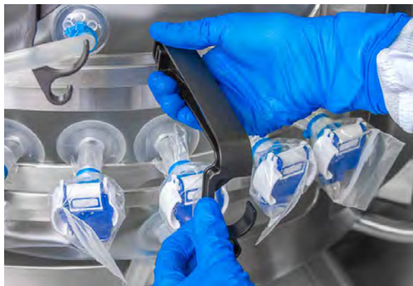
Figure 3.58. Attaching a probe clip.
