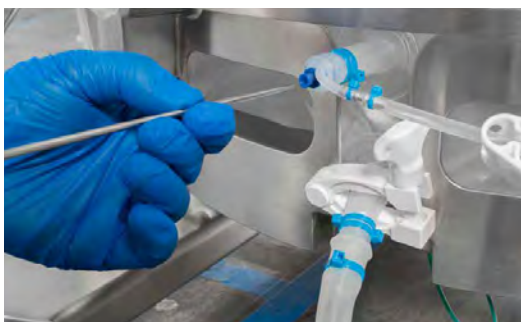
Figure 3.26. Inserting the RTD into the thermowell.
