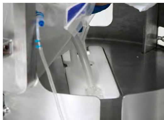
Figure 3.42. Replacing the guide plate.
