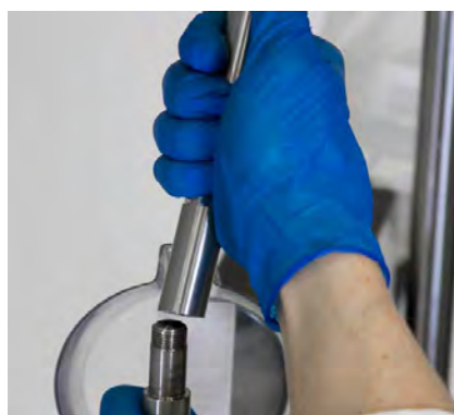
Figure 3.54. Connecting the upper drive shaft segment.
