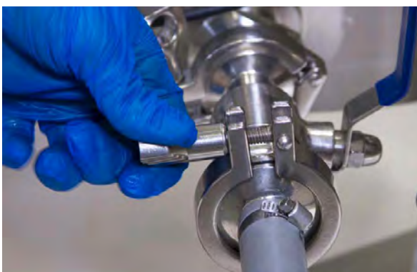
Figure 2.4. Attaching a TCU hose to the water jacket port.
