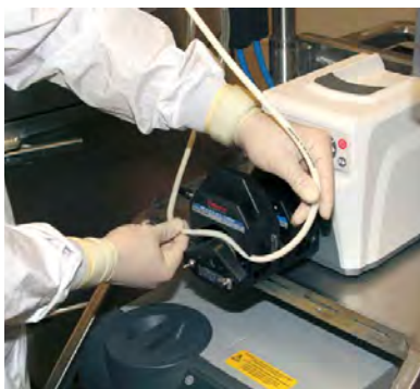
Figure 3.70. Loading pump tubing.
