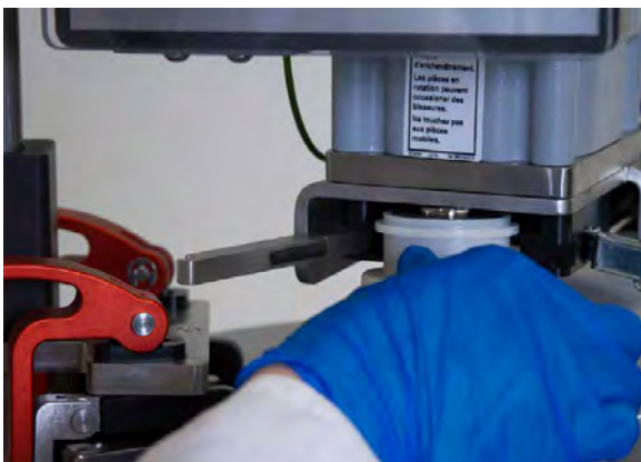
Figure 3.3. Inserting the bearing port.
