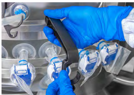
Figure 3.80. Attaching a probe clip.
