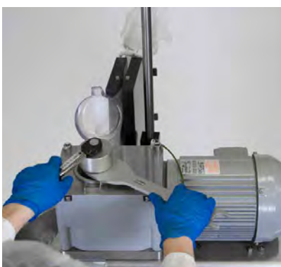
Figure 3.23. Tightening the cap.
