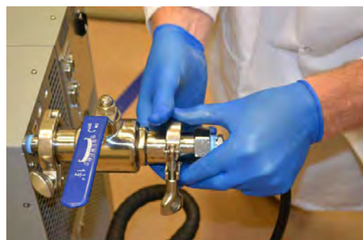
Figure 2.9. Attaching a clamp to a line.
