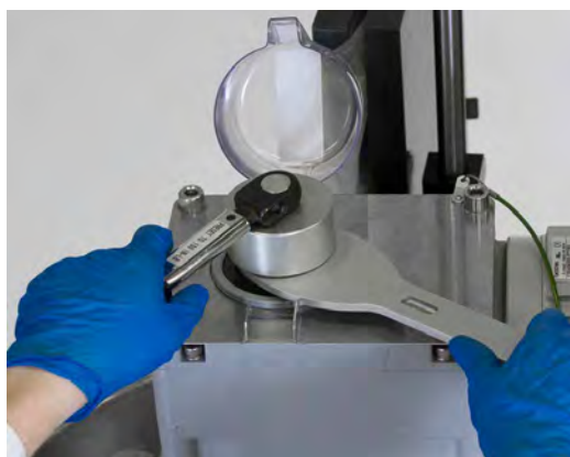
Figure 3.57. Tightening the cap with wrenches.
