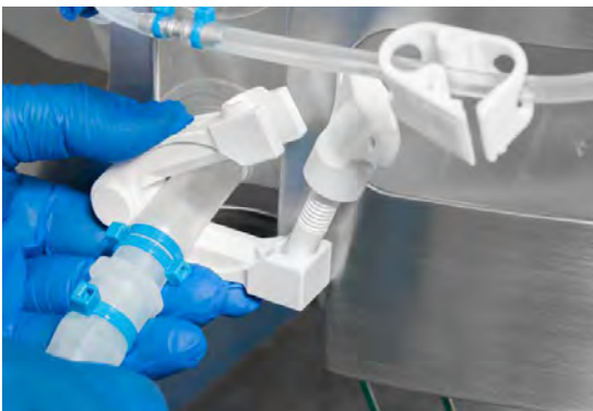
Figure 3.25. Closing bar clamp on drain line.
