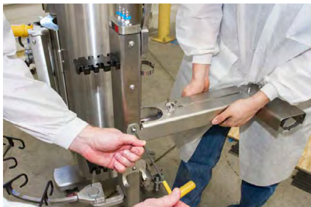
Figure 2.14. Attaching arm to cable management system.
