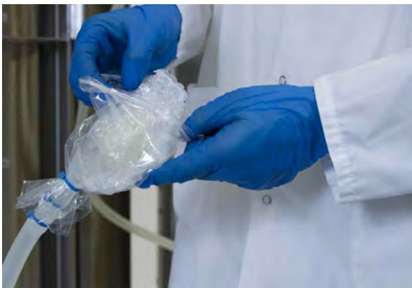
Figure 3.45. Sparge line and filter.
