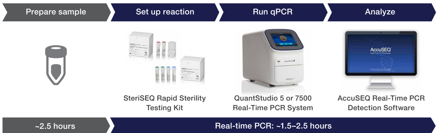
Figure 2. Workflow solution to support in-process and cell bank testing. The SteriSEQ kit is an integrated solution that includes analytical software reports for sterility testing during cell therapy manufacturing.
