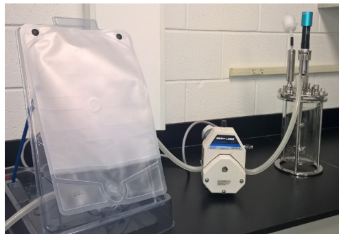
Figure 5. Transfer setup, with bioreactor connected to the Harvestainer BPC with pump.
