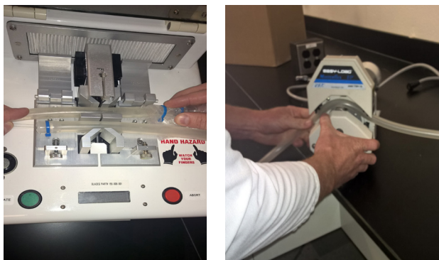
Figure 4. Connecting the lines and placing tubing in a pump.
