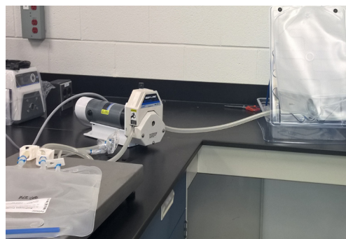
Figure 6. Drain setup, with the Harvestainer BPC connected to storage BPC with pump and scale.
