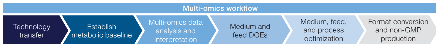
Figure 3. Multi-omics workflow. A typical multi-omics optimization project involves these phases and can evaluate up to 1,000 metabolites and 7,000 proteins.
