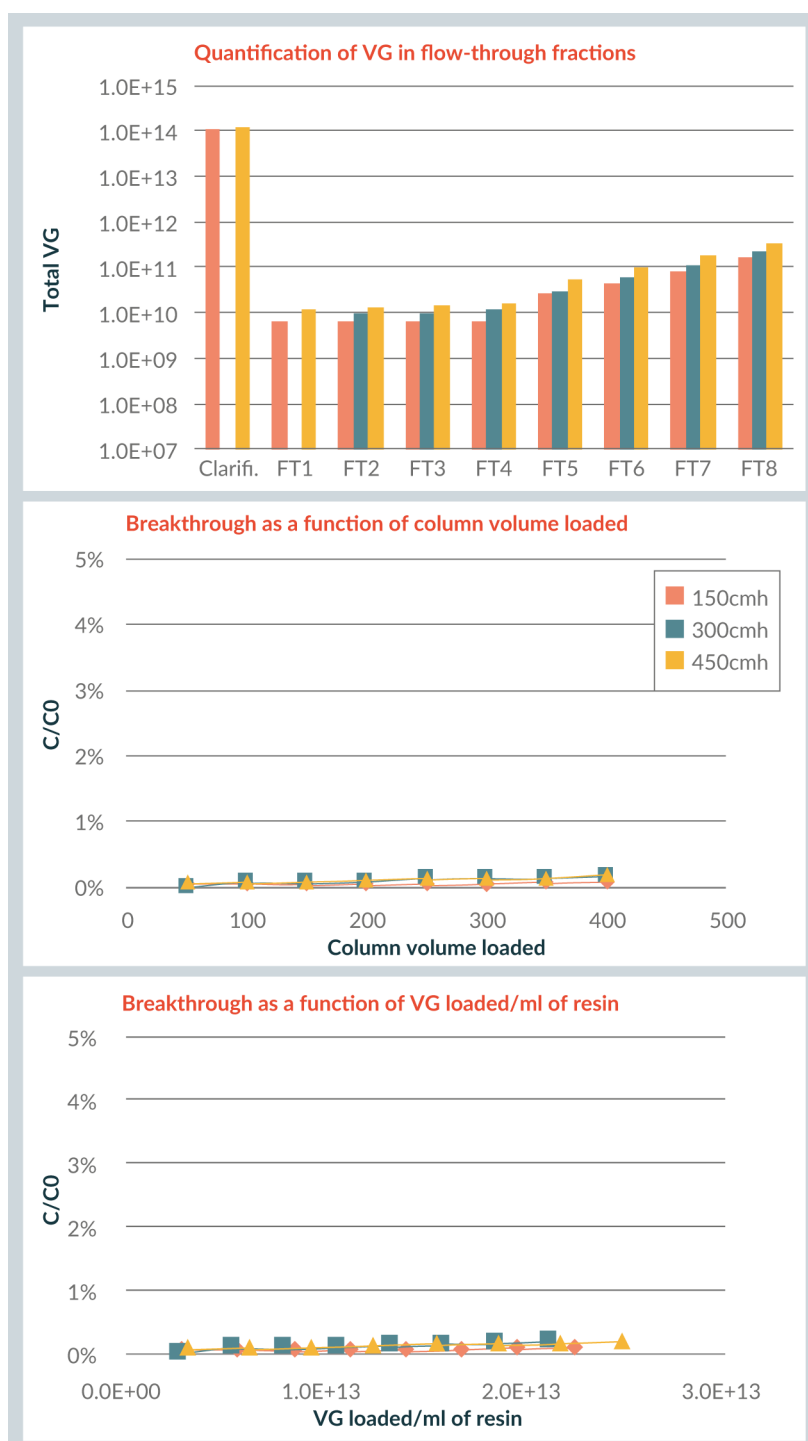
FIGURE 2 AAV8 breakthrough at different flow rates.
