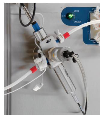
Figure 7. Post-column sensor pack with UV detector.
