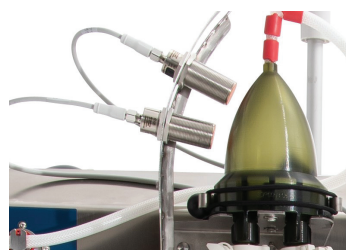
Figure 8. Bubble trap and level sensors.
