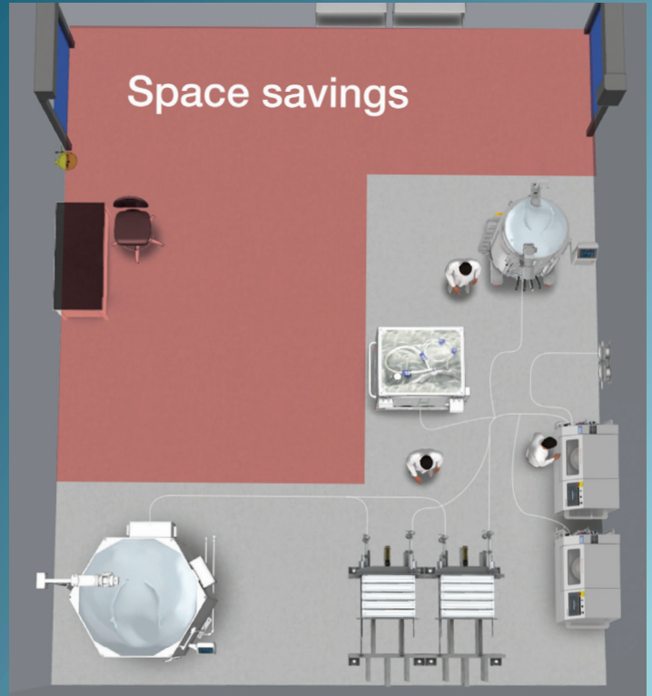
Figure 6b. Harvest suite layout for a 5,000 L bioreactor using DynaSpin with depth filtration.
