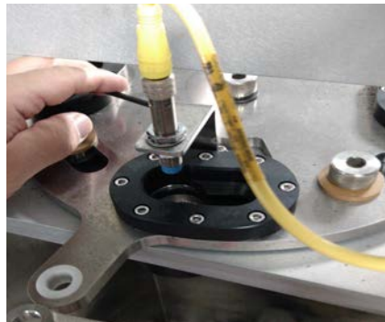
Figure 3.79. Replacing the two bolts to the sensor bracket.
