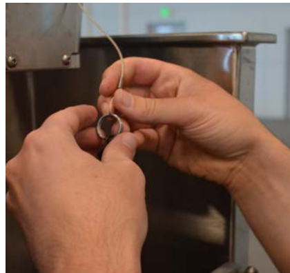
Figure 3.8. Removing quick-release pin from metal ring.
