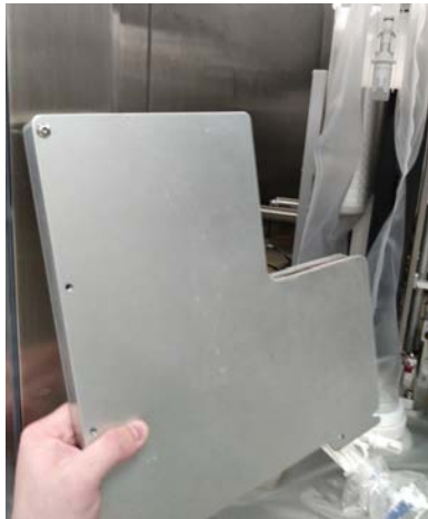
Figure 3.86. Removing the condenser heater from the heater mount.
