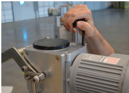
Figure 3.34. Securing one of the four bolts from the top of the motor assembly.
