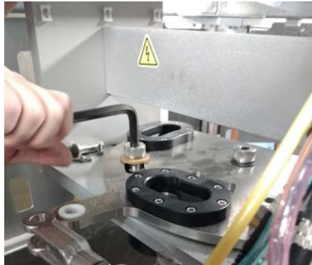
Figure 3.78. Removing bolts from the locking mechanism platform.
