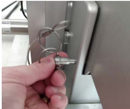
Figure 3.89. Replacing the lock pin.
