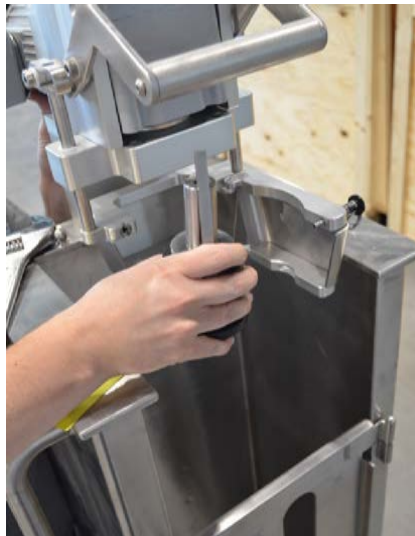
Figure 3.29. Replacing the hub locking mechanism at the bottom of the motor assembly.
