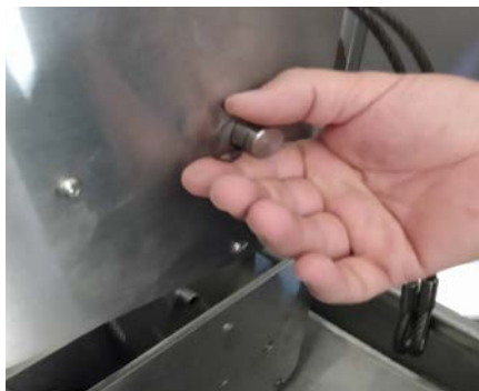
Figure 3.71. Replacing the c-clip and pin.
