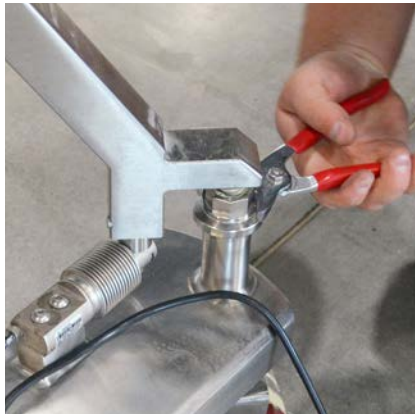
Figure 3.37. Twisting load cell lock-out nut clockwise.
