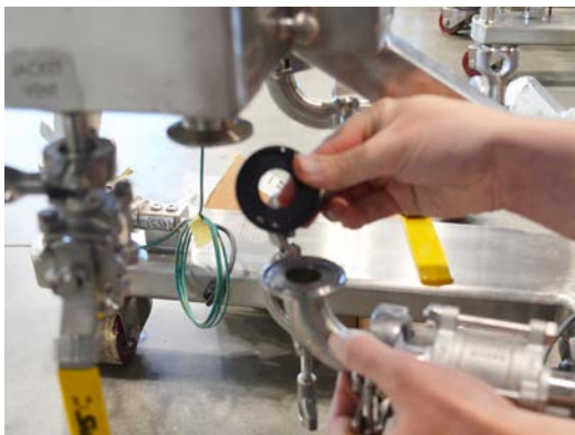
Figure 3.4. The rubber seal that is placed between the port and drain valve.
