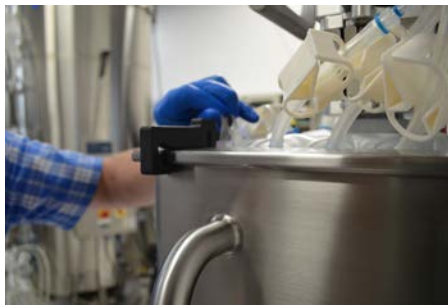
Figure 3.97. Pulling BPC tab over onto the tab holder sphere.
