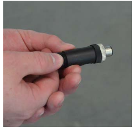
Figure 3.47. Screwing the last plastic piece to the tubing.
