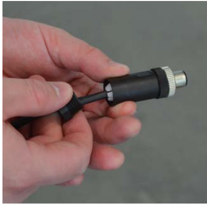
Figure 3.46. Sliding plastic piece up to tubing.
