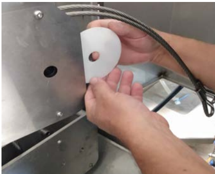
Figure 3.70. Replacing the front spacer to the pulley in the pulley assembly.
