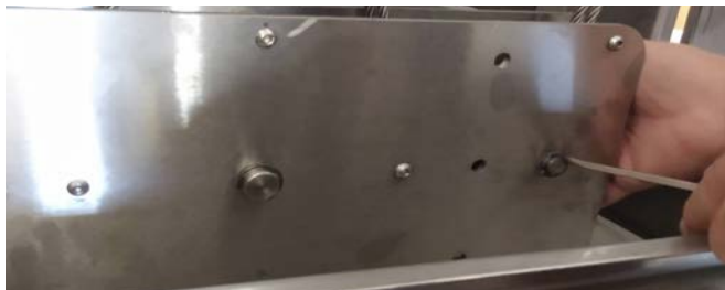
Figure 3.63. Removing the far right c-clip on the pulley assembly.
