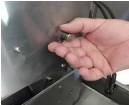
Figure 3.66. Removing the c-clip and pin.
