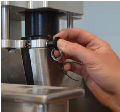
Figure 3.6. Pushing the release button on quick-release pin.
