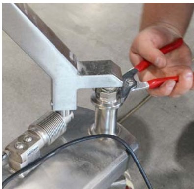
Figure 3.55. Twisting load cell lock-out nut counter-clockwise.
