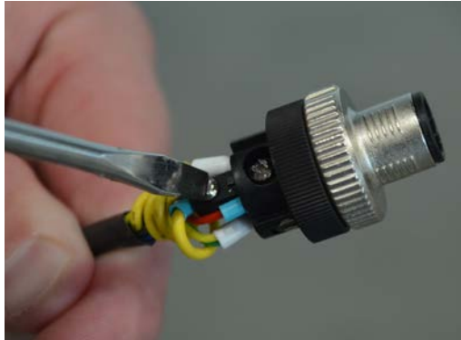
Figure 3.43. Tightening the screw to secure the wire into place.
