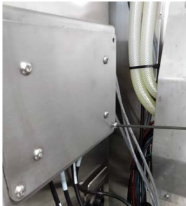
Figure 3.56. Four bolts on the summing block to remove.
