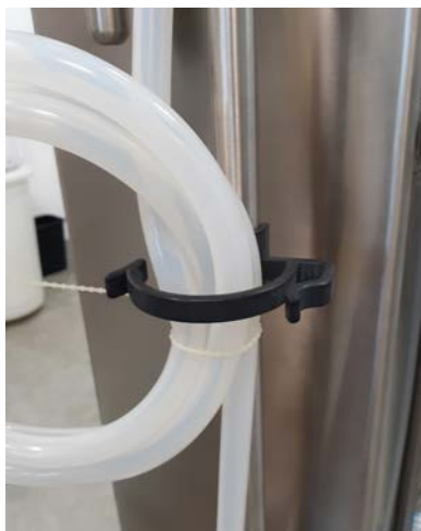
Figure 3.90. Tubing management system clipped to the handle bar.
