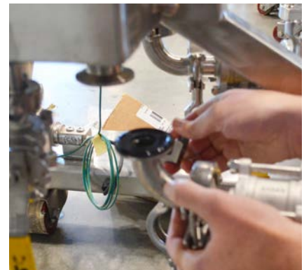
Figure 3.3. Removing drain valve from inlet/outlet port.
