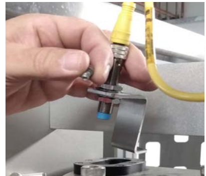
Figure 3.77. Detaching the sensor bracket.
