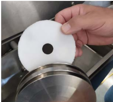
Figure 3.69. Replacing the back spacer and pulley.
