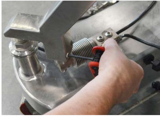
Figure 3.36. Loosening a bolt securing a load cell to a leg.
