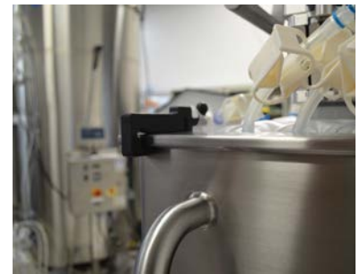
Figure 3.98. BPC tab on tab holder sphere.
