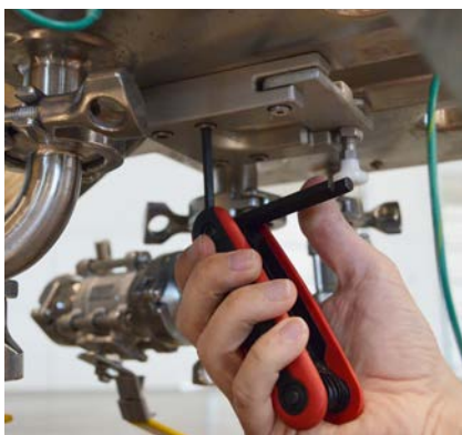
Figure 3.13. Removing four bolts from assembly bottom hub clamp.
