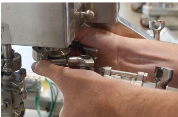
Figure 3.5. Attaching tri-clamp around inlet/outlet port and drain valve.
