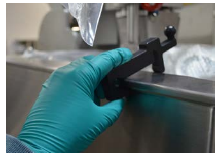
Figure 3.95. Sliding 500 L BPC tab holder into place.
