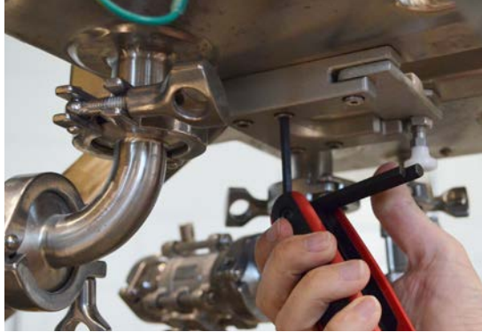
Figure 3.15. Replacing the four bolts to the assembly bottom hub clamp.
