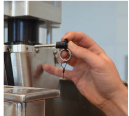
Figure 3.7. Removing the quick-release pin.
