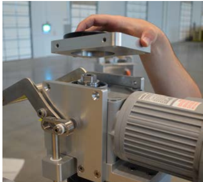
Figure 3.32. Replacing the top plate of the motor assembly.
