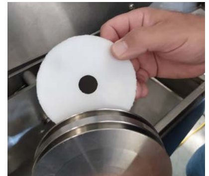
Figure 3.68. Removing the back spacer and pulley from the pulley assembly.
