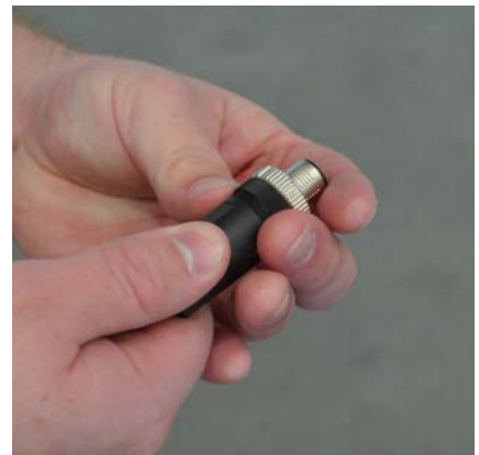
Figure 3.45. Screwing the end of the plastic tube to the end of the pin-out connector.
