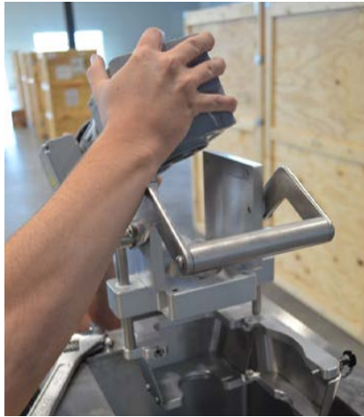
Figure 3.28. Replacing the motor from the motor assembly.
