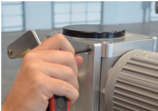
Figure 3.17. Removing the top two bolts from the side of the motor assembly.
