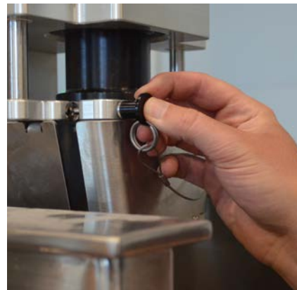
Figure 3.12. Replacing the quick-release pin.
