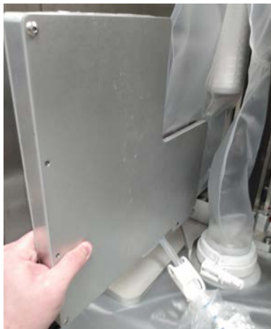
Figure 3.87. Replacing the condenser heater from the heater mount.
