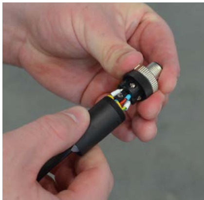
Figure 3.44. Sliding plastic tubing over wiring.
