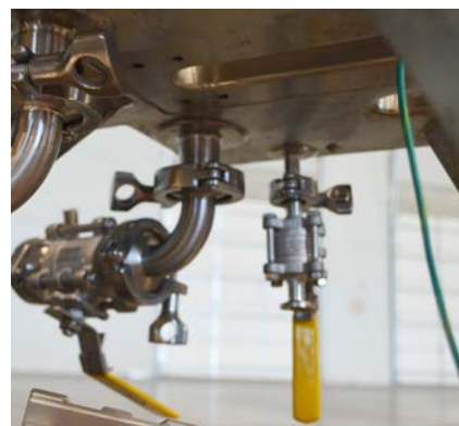
Figure 3.14. Removing the assembly bottom hub clamp.
