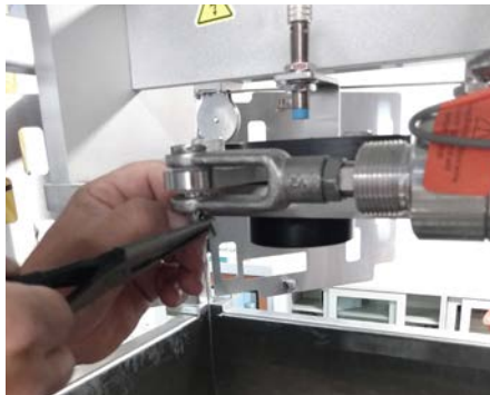
Figure 3.81. Replacing locking pin to locking cylinder arm.
