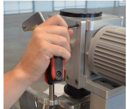
Figure 3.33. Securing the top two bolts from side of motor assembly.
