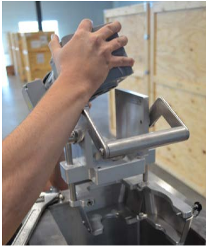
Figure 3.21. Removing the motor from the motor assembly.
