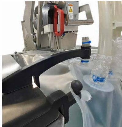
Figure 3.92. 500 L foam probe holder.
