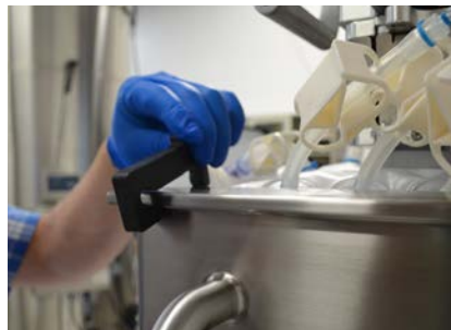
Figure 3.94. Sliding 50 L BPC tab holder into place.
