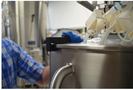
Figure 3.96. BPC tab holder in place.
