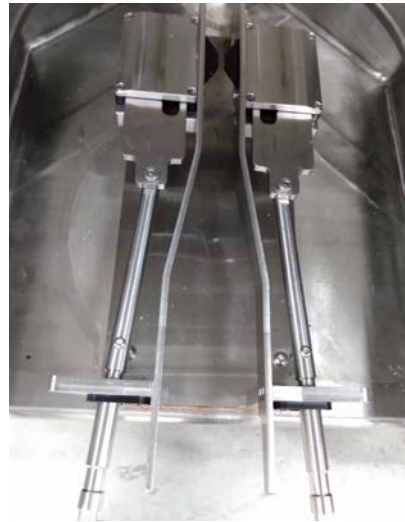
Figure 3.83. Replacing bottom hub clamp assembly.
