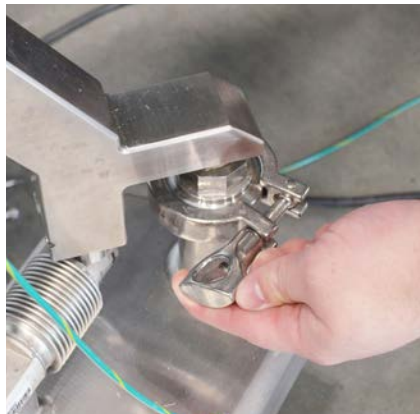
Figure 3.35. Removing the wing nut tri-clamp.
