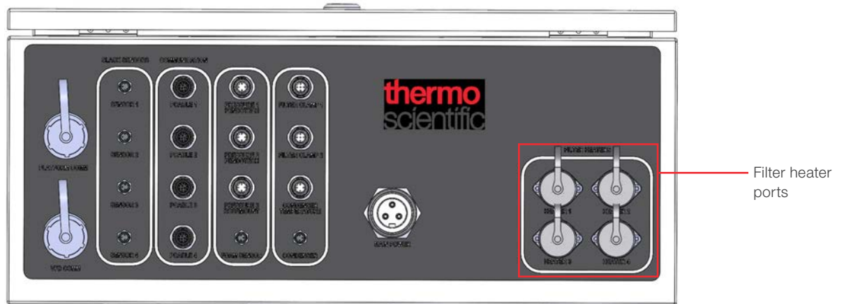
Figure 3.85. VFD electrical box and filter heater ports.
