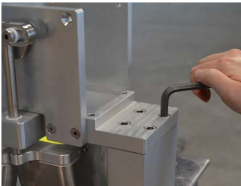
Figure 3.22. Loosening the bolts on top of the motor mount.
