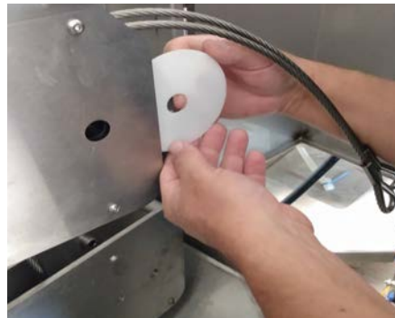
Figure 3.67. Removing the front spacer from the pulley.
