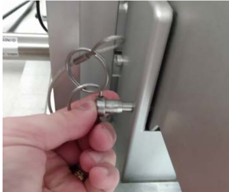
Figure 3.84. Removing the lock pin.
