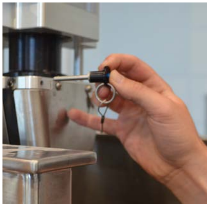
Figure 3.11. Pushing the release button on quick-release pin.
