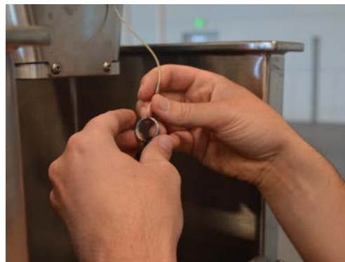
Figure 3.10. Attaching new latch pin to the ring.
