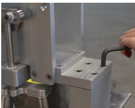
Figure 3.24. Securing the bolts on top of the motor mount.
