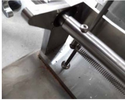
Figure 3.82. Removing one of six bolts from bottom hub clamp assembly.
