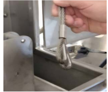
Figure 3.65. Removing the end of the cables from the pulley assembly.
