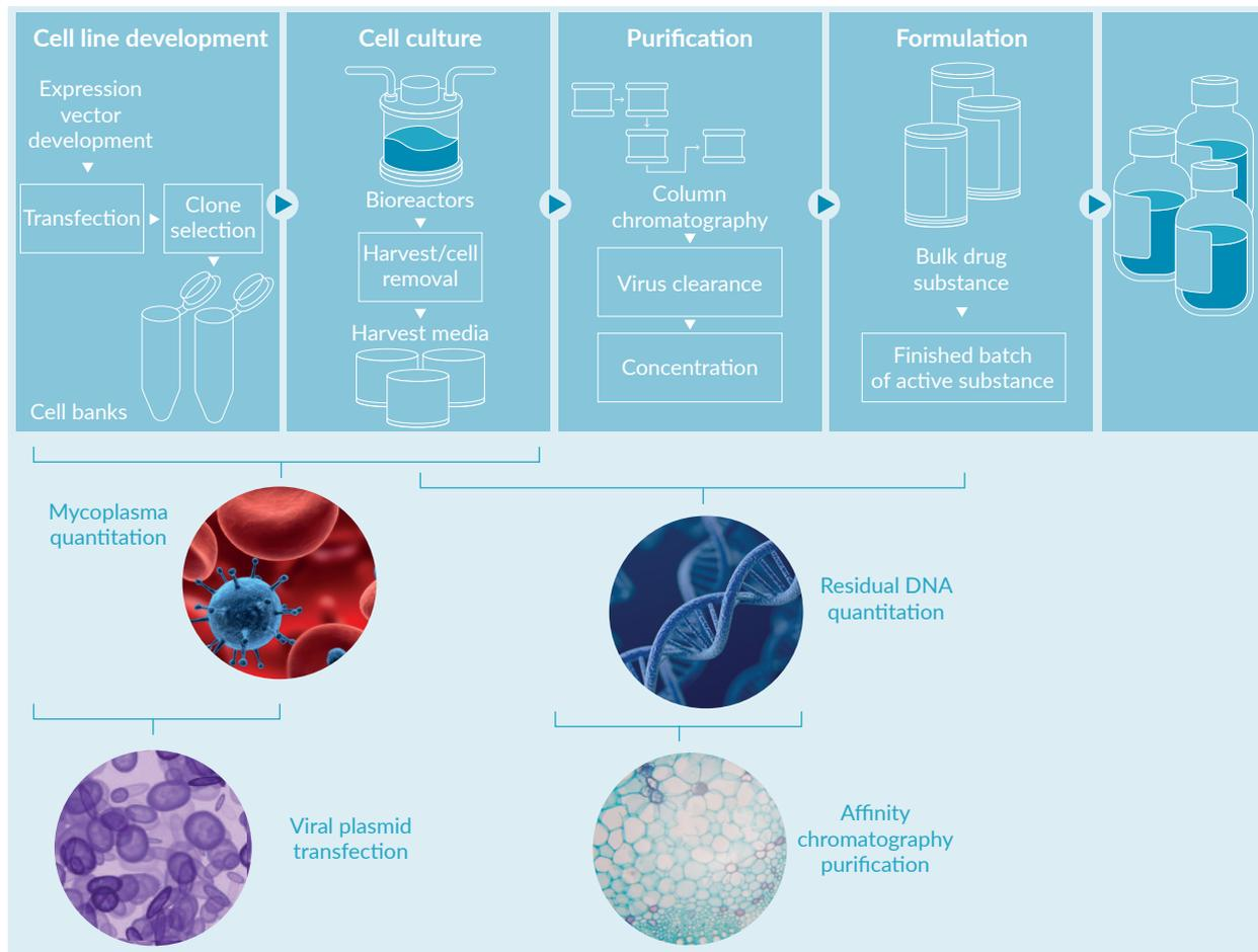
The upstream processes include cell line development, cell culture, and viral harvest. The downstream processes include purification, formulation, and filling.
