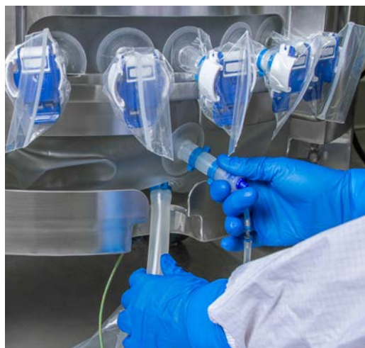
Figure 3.38. Drain/sampling line extension.
