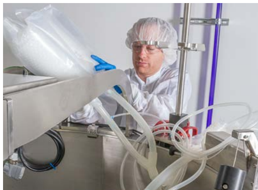
Figure 3.65. Placing linesets over tank edge.
