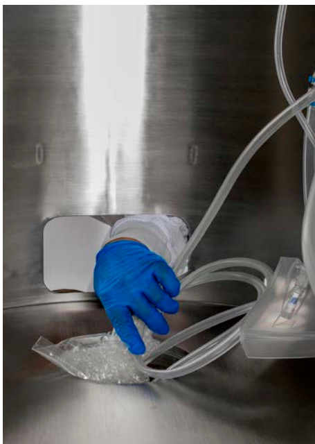
Figure 3.35. Sparge line insertion.
