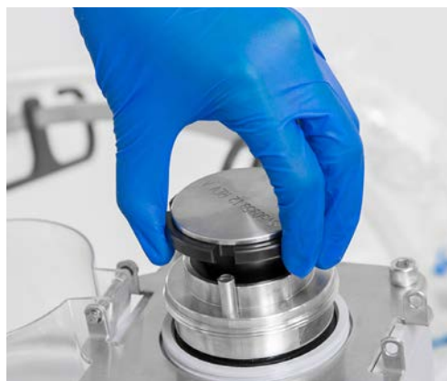
Figure 3.51. Drive shaft head aligned.
