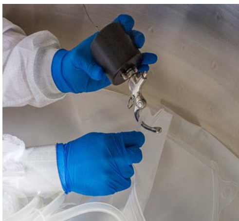
Figure 3.61. Connecting tabs to BPC lift.
