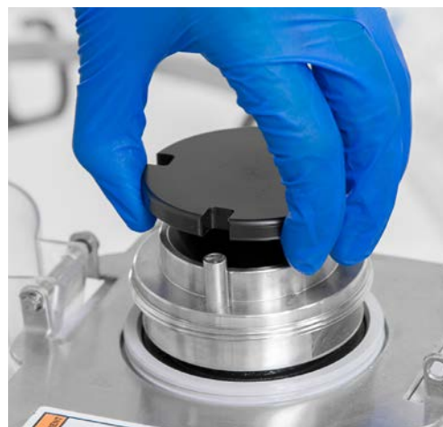
Figure 3.19. Drive shaft head aligned.
