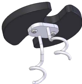
Figure 1.22. Figure 1.22. Sparge line support.
