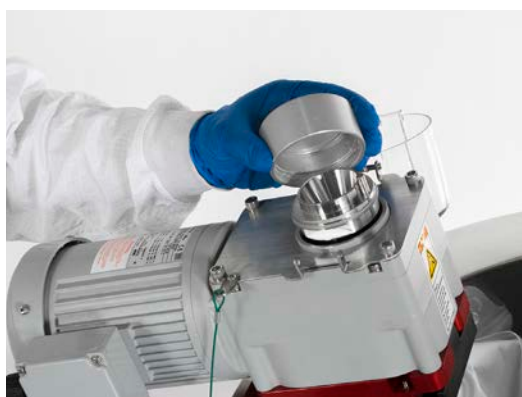
Figure 3.43. Latch pin removal.
