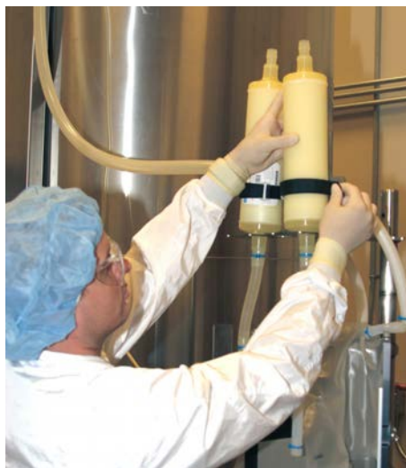
Figure 3.81. Securing vent filters.
