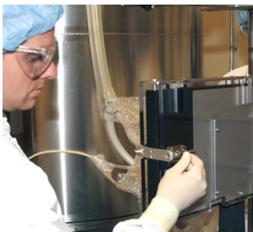
Figure 3.78. Opening the chiller plate doors.
