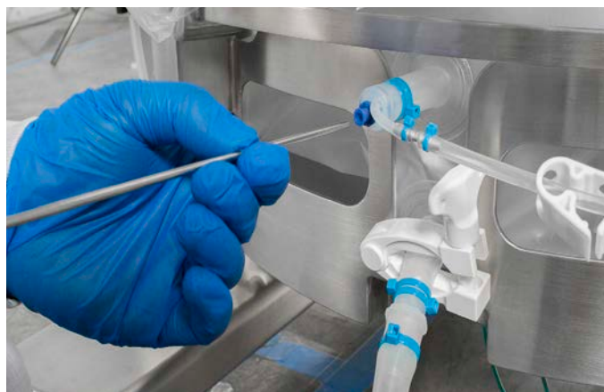
Figure 3.56. Temperature sensor insertion.
