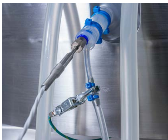
Figure 3.107. Grounding cable connected
