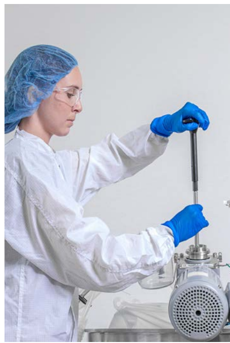
Figure 3.17. Twisting drive shaft to aid insertion.
