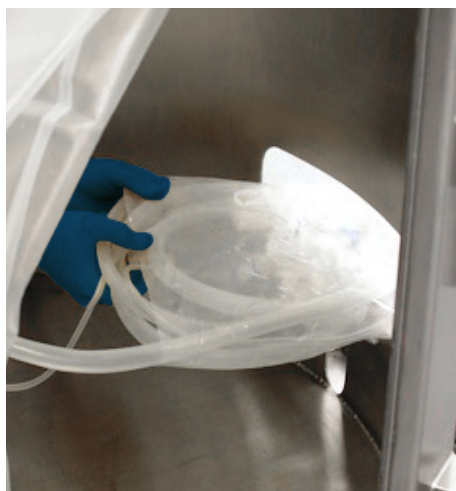
Figure 3.37. Drain/sampling line set insertion.
