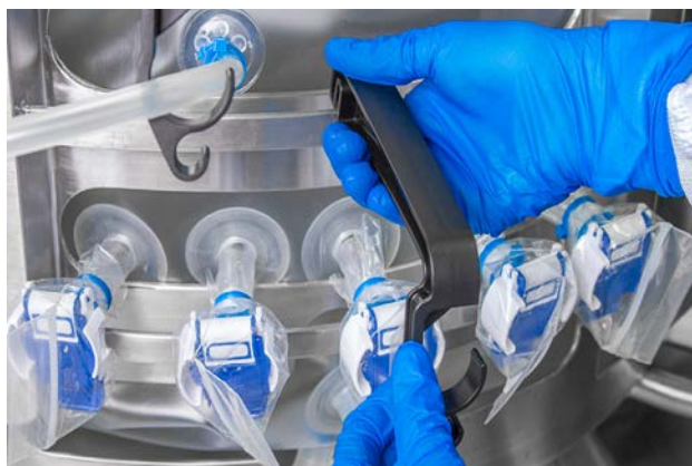
Figure 3.117. Attaching plastic probe clip.
