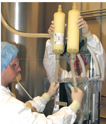
Figure 3.80. Placing vent filters.
