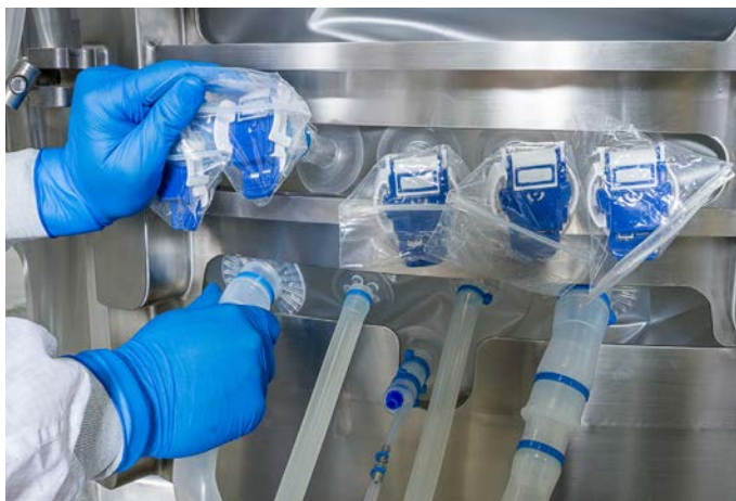
Figure 3.103. Aseptic port alignment.
