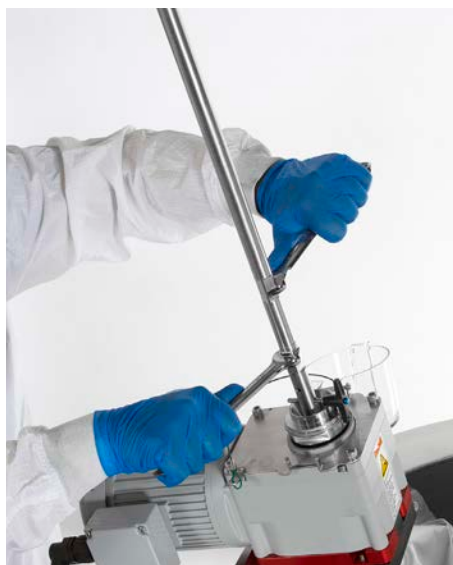
Figure 3.49. Tightening of shaft connections.
