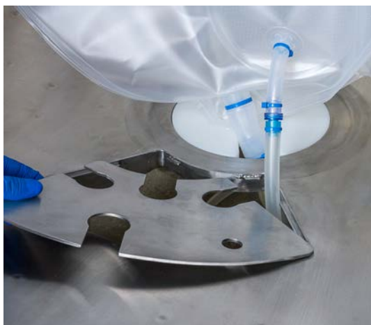
Figure 3.73. Drilled hole sparger line.
