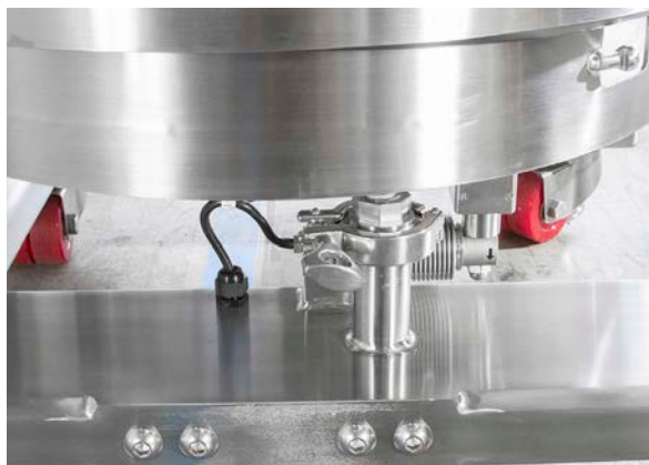
Figure 1.20. Load cell location.
