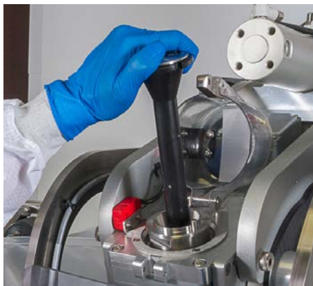
Figure 3.99. Insertion of the drive shaft. Figure 3.100. Engaging the bearing port.
