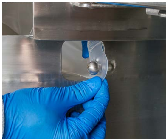
Figure 3.75. Securing the container tab on the pin.
