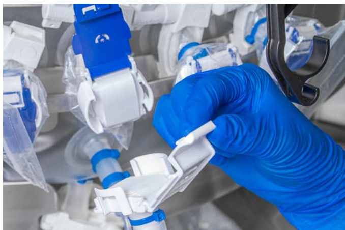
Figure 3.114. Opening protective cover pull tab on lineset.
