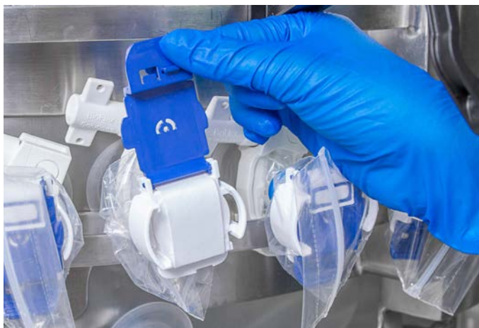
Figure 3.113. Opening protective cover pull tab on port.
