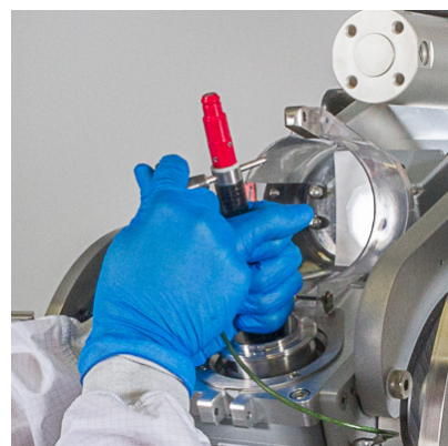
Figure 3.93. Using the latch pin.
