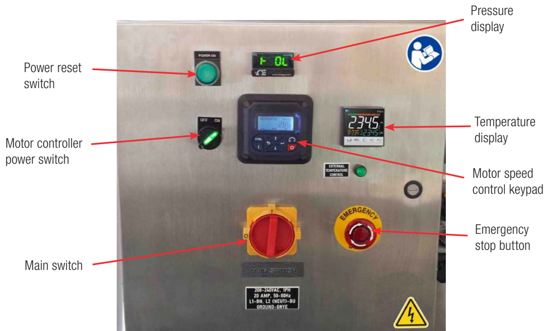
Figure 4.21. Front view of the E-Box for 50–2,000 L S.U.B.s.
