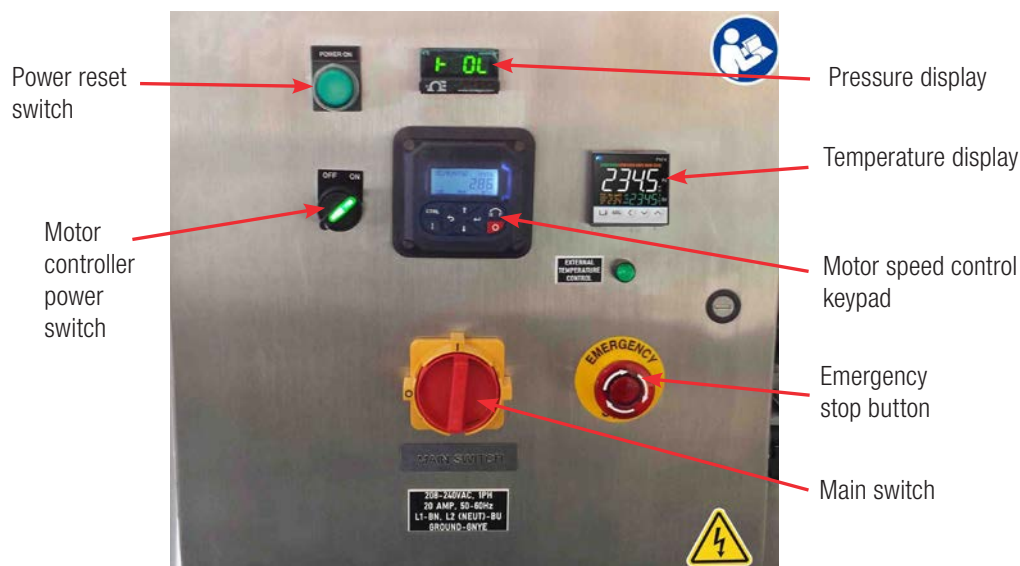
Figure 3.121. Front view of E-Box for 50–2,000 L S.U.B.s.
