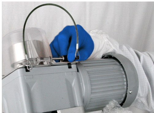
Figure 3.22. Replacing and latching cover.
