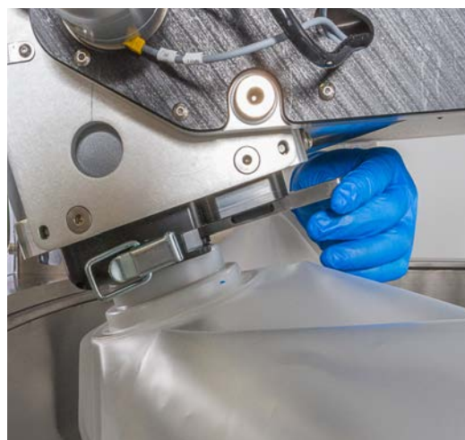
Figure 3.64. Closing and latching door.
