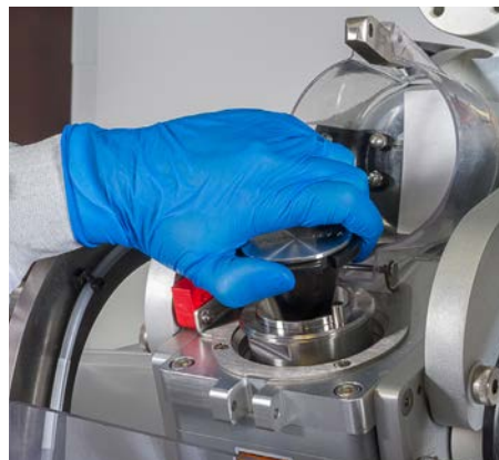
Figure 3.99. Insertion of the drive shaft. Figure 3.100. Engaging the bearing port.
