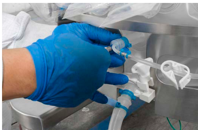
Figure 3.57. Securing temperature sensor.
