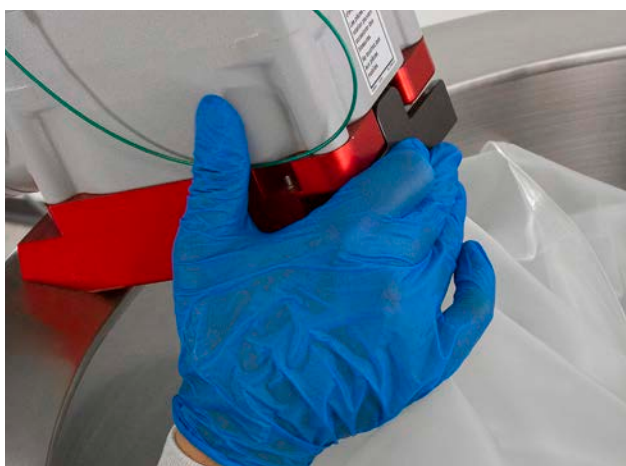
Figure 3.34. Door clamped shut.
