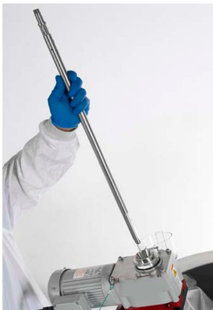
Figure 3.46. Inserting lower section.
