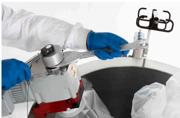
Figure 3.52. Tightening motor cap with wrenches.
