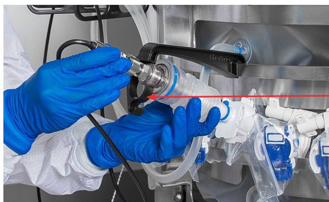
Figure 3.120. Positioning probe clip.
