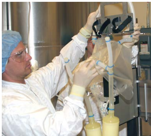
Figure 3.79. Routing gas inlet lines.
