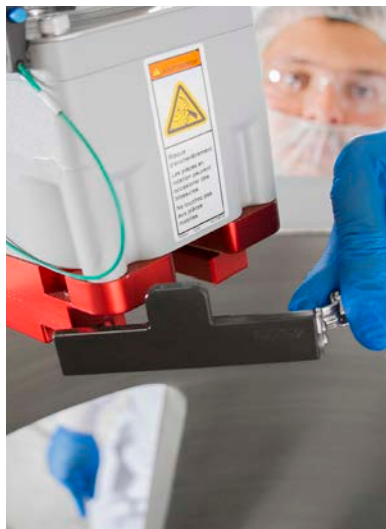
Figure 3.29. Close-up of bearing receiver clamp.
