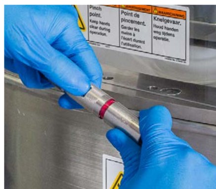
Figure 3.95. Sliding sleeve exposing red "not locked" indicator.
