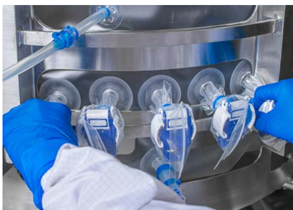
Figure 3.55. Aseptic connector port alignment.
