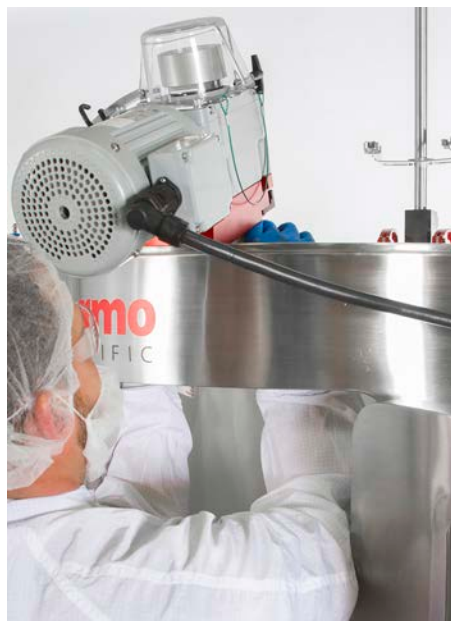
Figure 3.31. Bearing port orientation.
