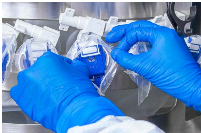
Figure 3.112. Removing plastic covering from connector.
