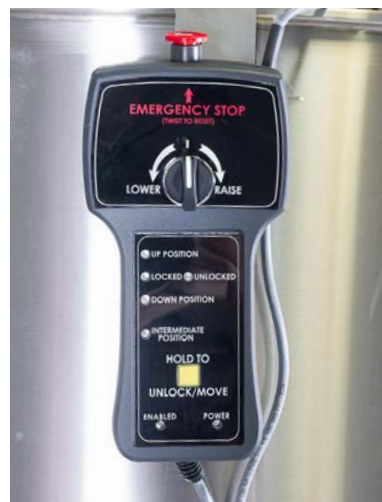
Figure 1.17. Handheld controller for motor lifts.
