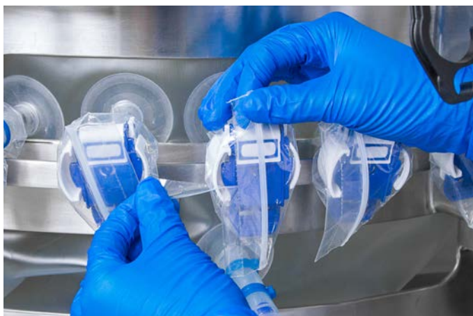
Figure 3.111. Pulling the tear strip.
