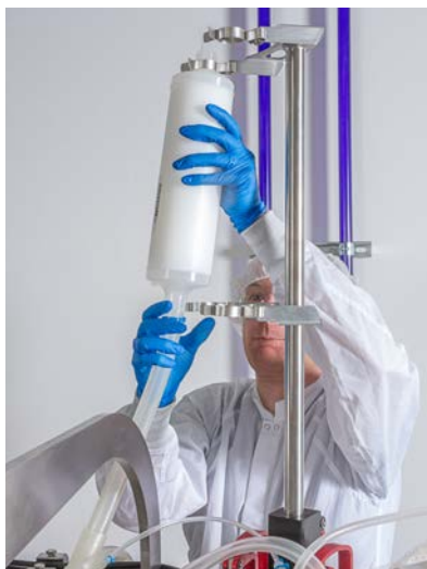
Figure 3.66. Clipping filter to holder.
