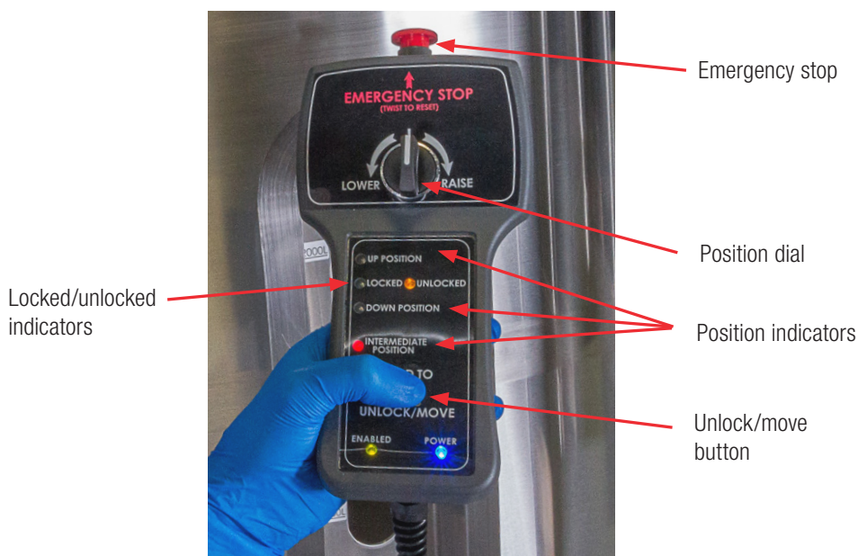
Figure 2.8. Handheld controller for motor lifts.
