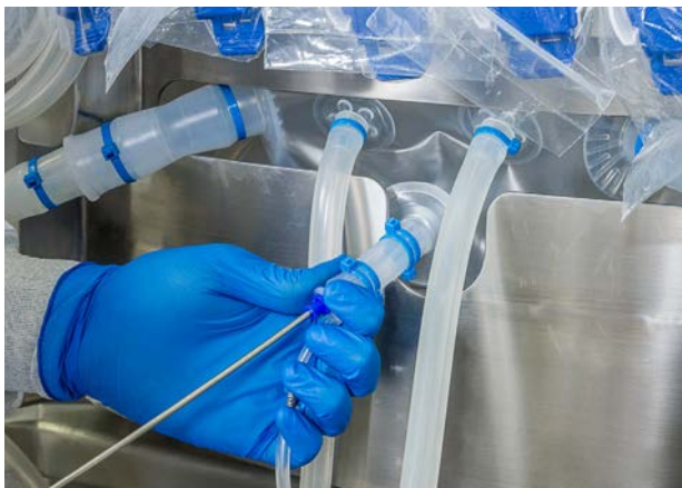
Figure 3.106. Insertion of the RTD into the thermowell.
