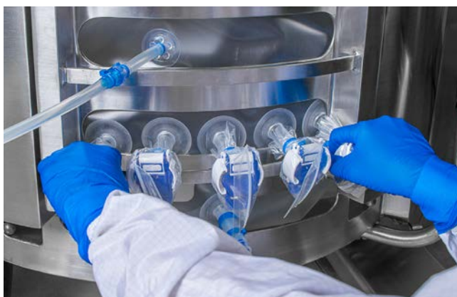
Figure 3.12. Aseptic connector alignment.
