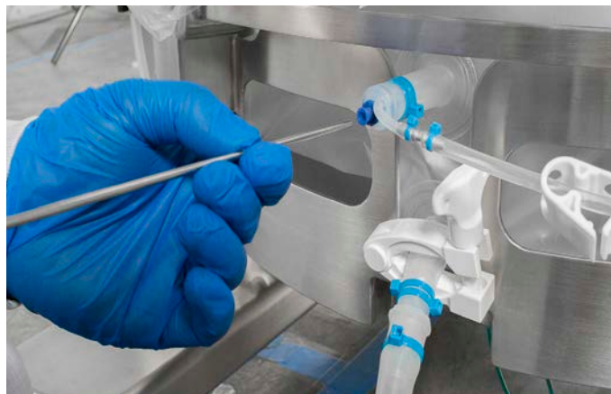
Figure 3.56. Temperature sensor insertion.
