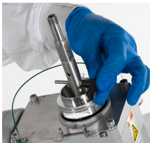
Figure 3.47. Latch pin in shaft.
