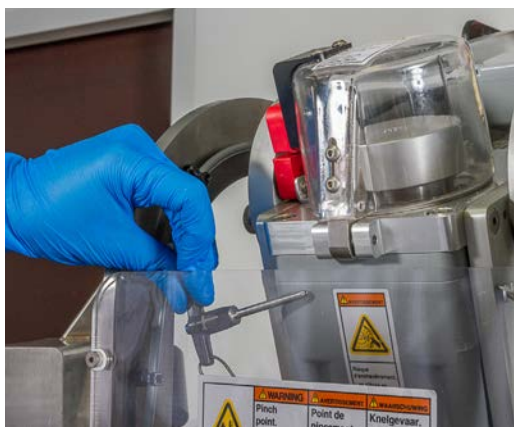
Figure 3.90. Removing latch pin.
