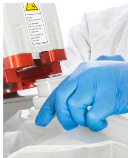
Figure 3.3. Bearing port insertion.
