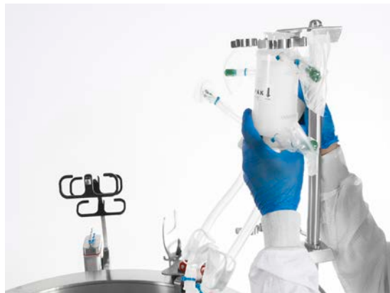
Figure 3.54. Extended dual filter bracket.
