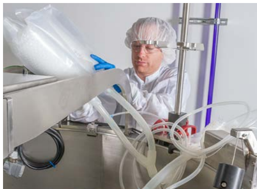
Figure 3.65. Placing linesets over tank edge.
