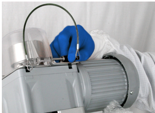
Figure 3.22. Replacing and latching cover.
