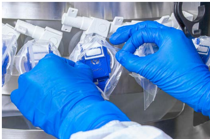
Figure 3.112. Removing plastic covering from connector.
