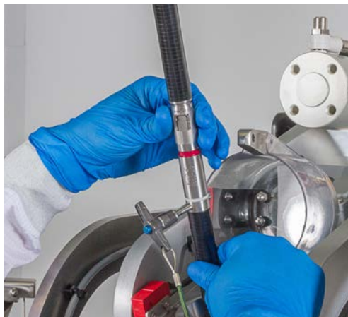
Figure 3.97. Red indicator ring exposed.
