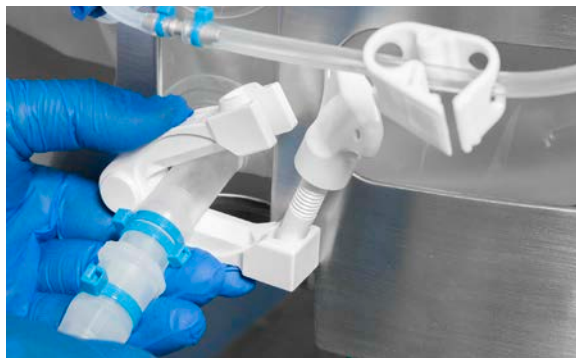
Figure 3.25. Bar clamp installation.
