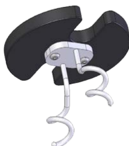
Figure 2.6. Sparge line support.
