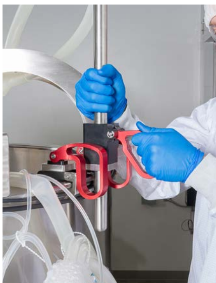
Figure 3.68. Raising the vent holder bracket.
