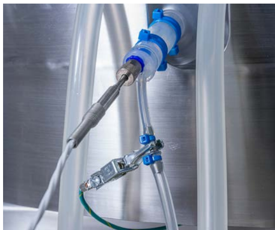
Figure 3.107. Grounding cable connected
