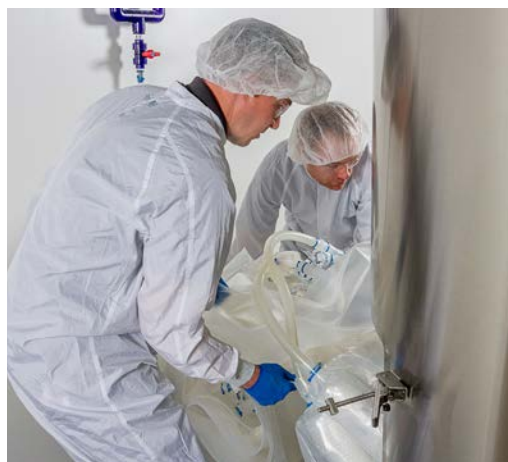
Figure 3.60. Loading the BPC.
