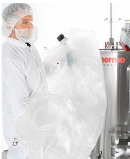
Figure 3.1. BPC removed from protective double polybags.
