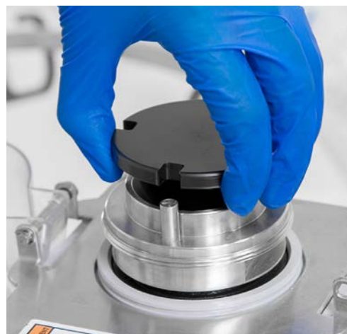
Figure 3.19. Drive shaft head aligned.
