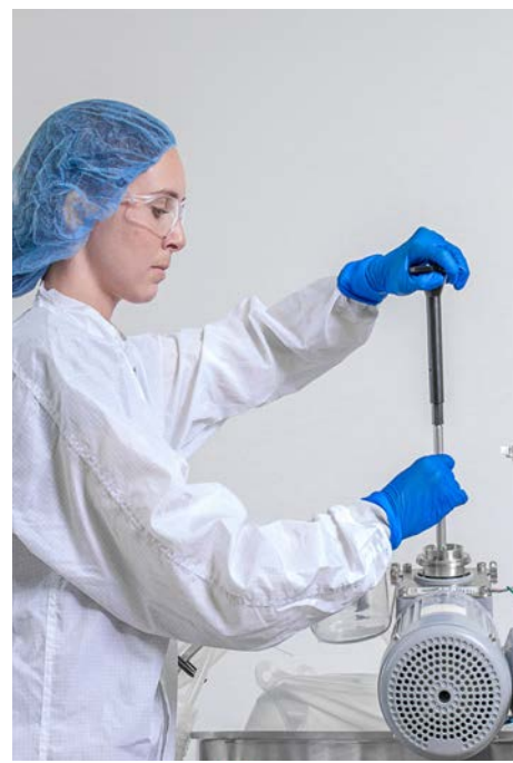
Figure 3.17. Twisting drive shaft to aid insertion.
