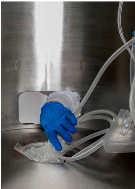
Figure 3.35. Sparge line insertion.
