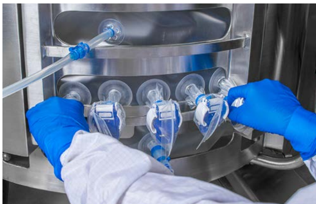
Figure 3.12. Aseptic connector alignment.
