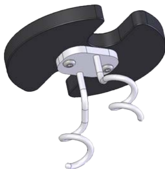
Figure 1.22. Figure 1.22. Sparge line support.
