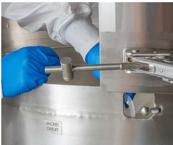
Figure 3.74. Pulling the container tab toward the pin.
