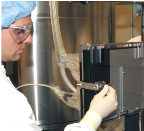
Figure 3.78. Opening the chiller plate doors.
