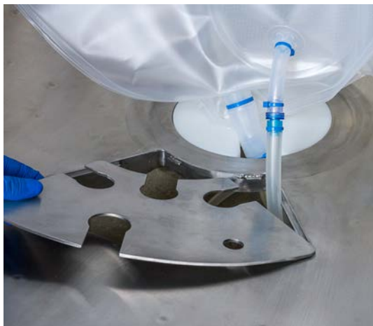
Figure 3.73. Drilled hole sparger line.
