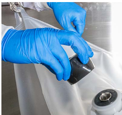
Figure 3.62. Removing the bearing port cap.
