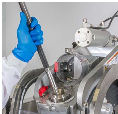
Figure 3.92. Insertion of the lower section of the drive shaft.
