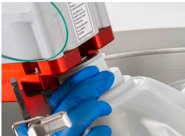
Figure 3.33. Bearing port in receiver.
