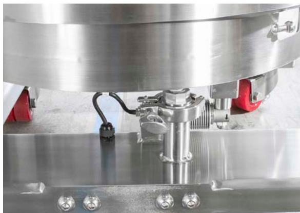
Figure 1.20. Load cell location.
