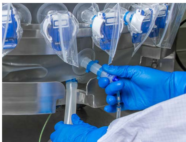
Figure 3.6. Drain line and port setup.
