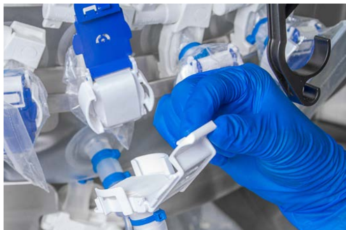
Figure 3.114. Opening protective cover pull tab on lineset.
