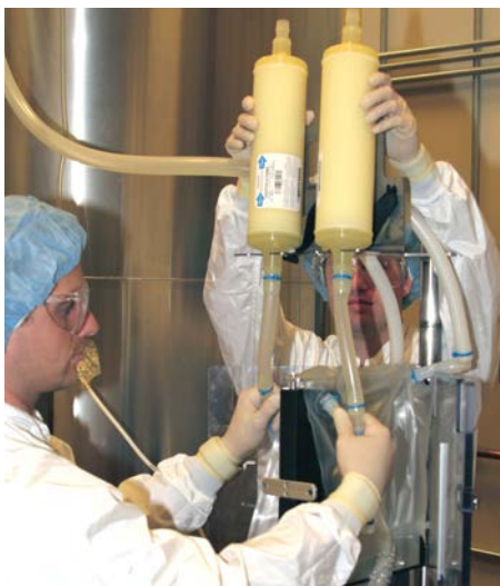
Figure 3.80. Placing vent filters.
