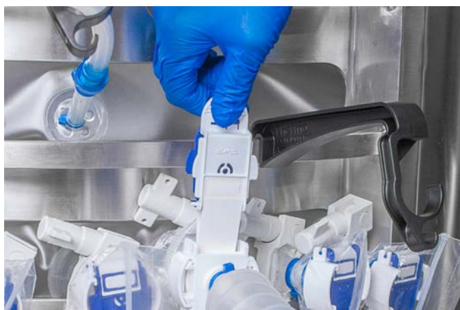
Figure 3.116. Pulling tabs to remove paper membranes.
