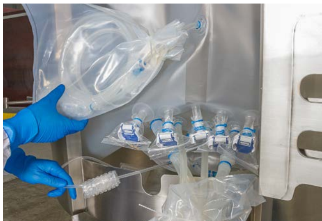
Figure 3.70. Feeding lines through the front access door.
