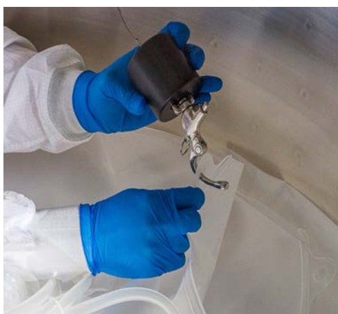
Figure 3.61. Connecting tabs to BPC lift.
