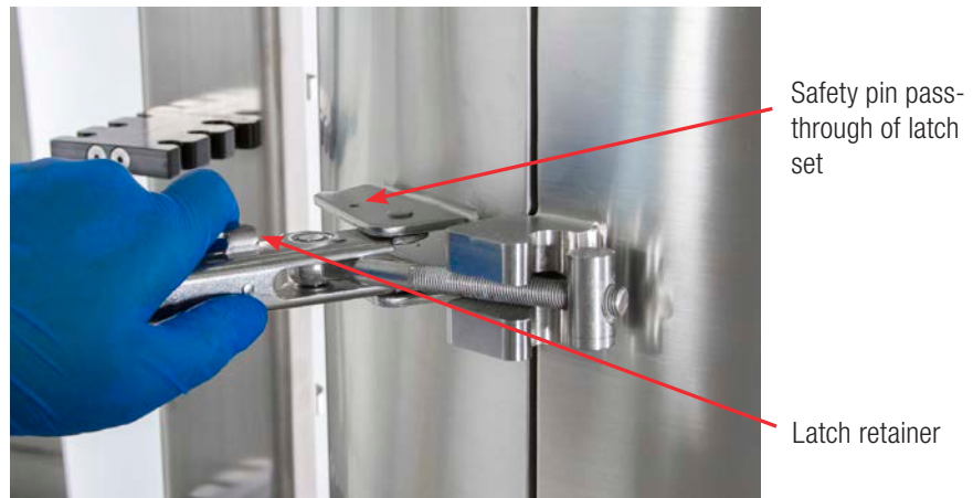
Figure 3.58. Latching the access door.
