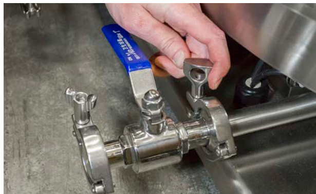
Figure 2.4. Attaching water jacket port using tri-clamp.
