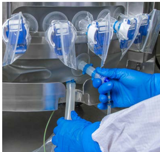
Figure 3.38. Drain/sampling line extension.
