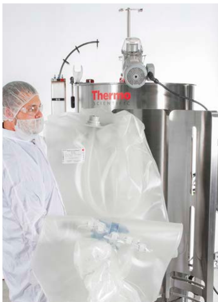
Figure 3.30. BPC in protective polybags.
