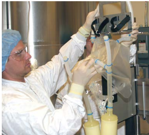
Figure 3.79. Routing gas inlet lines.
