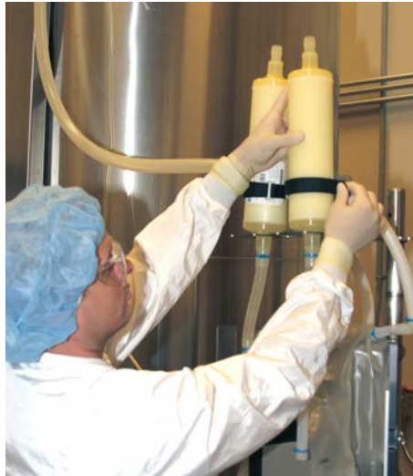
Figure 3.81. Securing vent filters.
