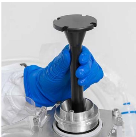
Figure 3.18. Preparing to engage impeller.
