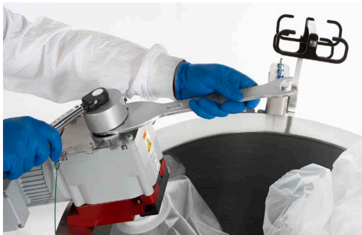
Figure 3.52. Tightening motor cap with wrenches.
