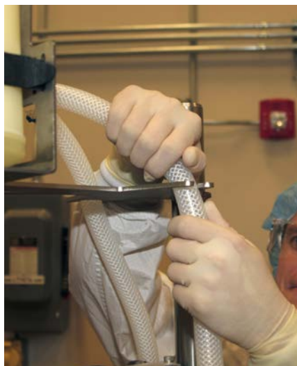
Figure 3.85. Clipping gas lines into place.
