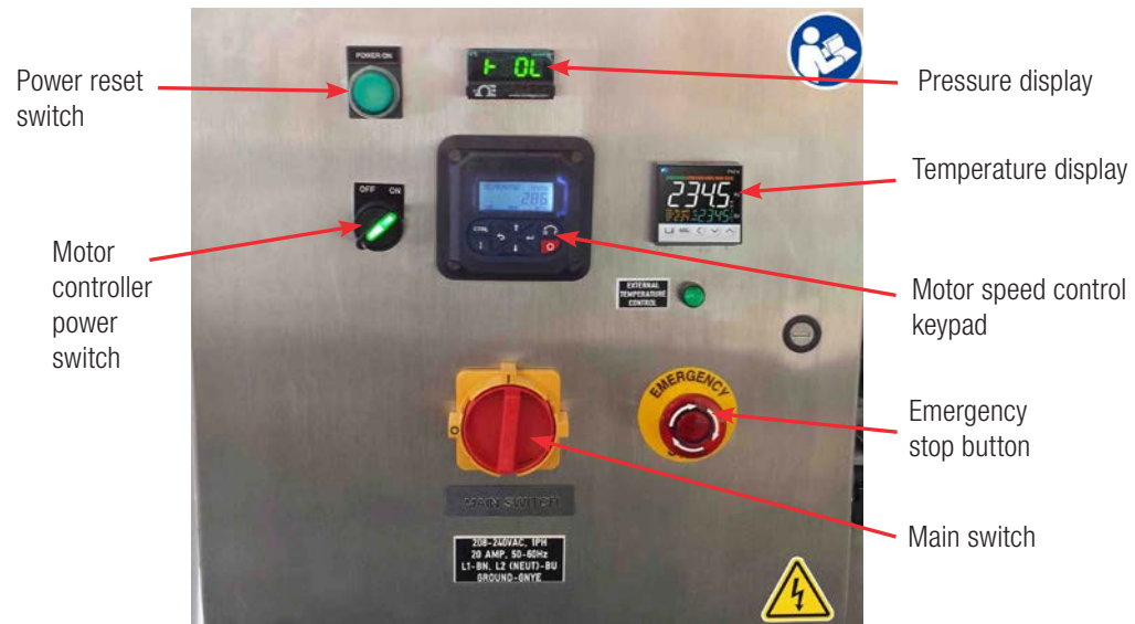
Figure 3.121. Front view of E-Box for 50–2,000 L S.U.B.s.
