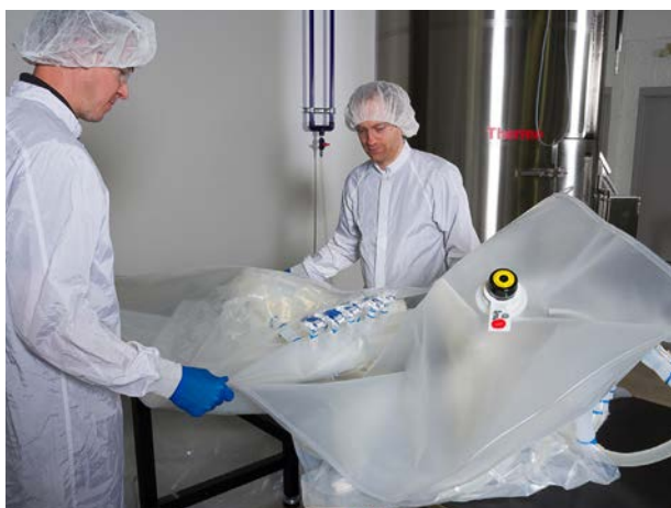
Figure 3.59. Removing the BPC from polybags.
