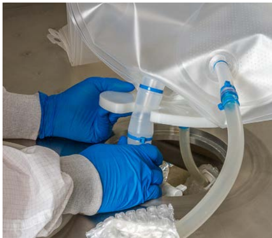
Figure 3.72. Drain line support.
