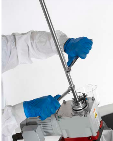
Figure 3.49. Tightening of shaft connections.
