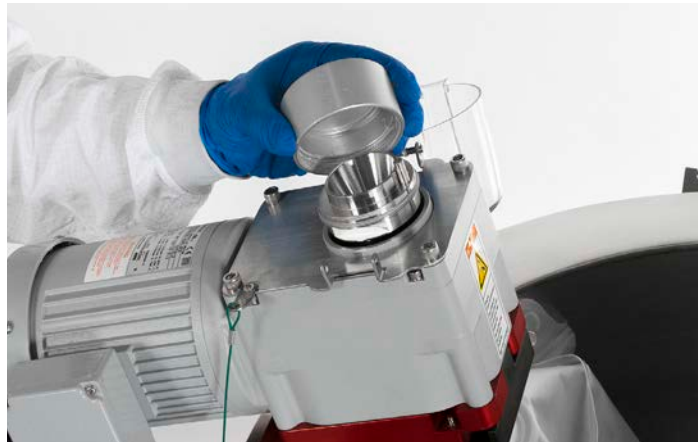
Figure 3.15. Removing the motor cap.
