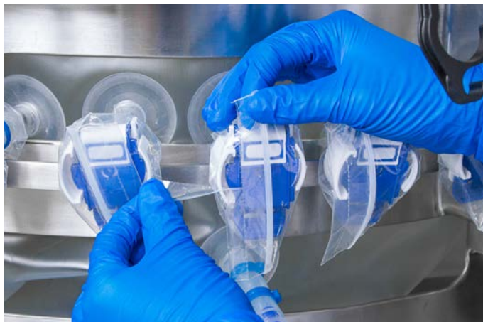
Figure 3.111. Pulling the tear strip.
