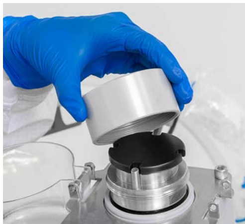
Figure 3.20. Replacing motor cap.
