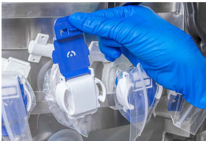
Figure 3.113. Opening protective cover pull tab on port.
