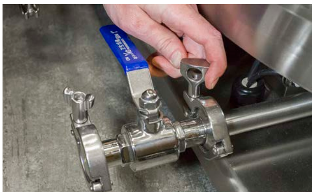
Figure 2.4. Attaching water jacket port using tri-clamp.
