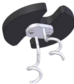
Figure 2.6. Sparge line support.
