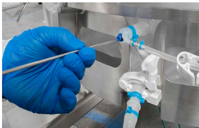
Figure 3.56. Temperature sensor insertion.
