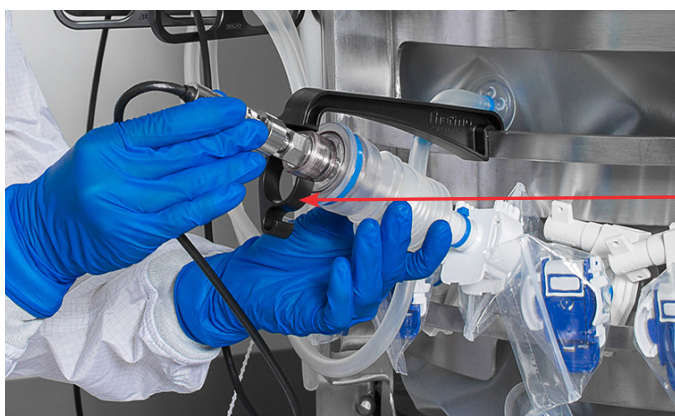
Figure 3.120. Positioning probe clip.
