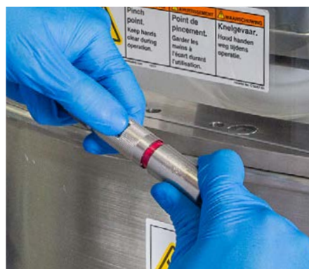
Figure 3.95. Sliding sleeve exposing red "not locked" indicator.
