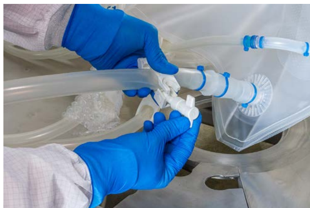
Figure 3.71. Clamping bottom drain line.
