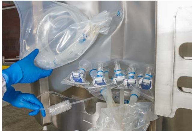
Figure 3.70. Feeding lines through the front access door.
