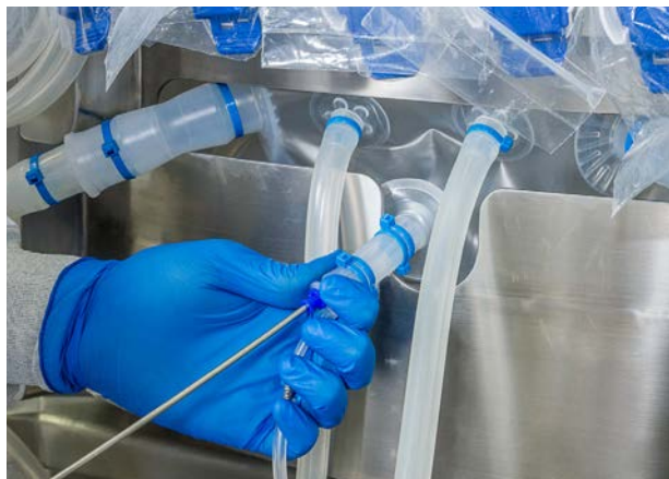
Figure 3.106. Insertion of the RTD into the thermowell.
