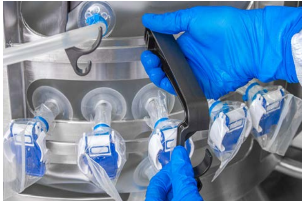
Figure 3.117. Attaching plastic probe clip.
