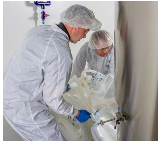
Figure 3.60. Loading the BPC.
