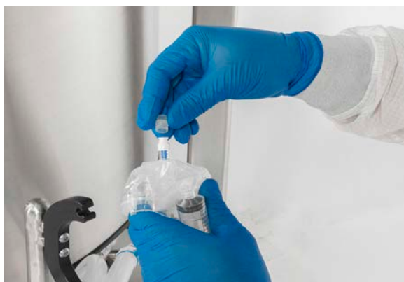
Figure 3.124. Removal of dust cover from SmartSite.
