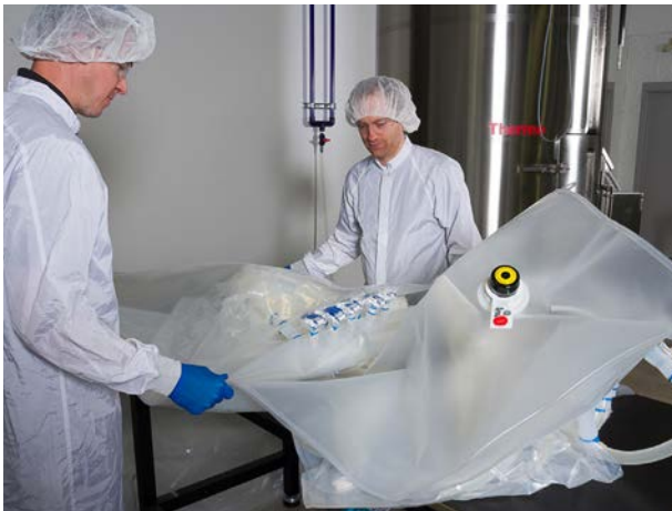
Figure 3.59. Removing the BPC from polybags.
