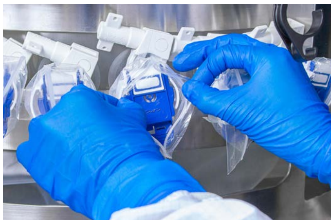
Figure 3.112. Removing plastic covering from connector.
