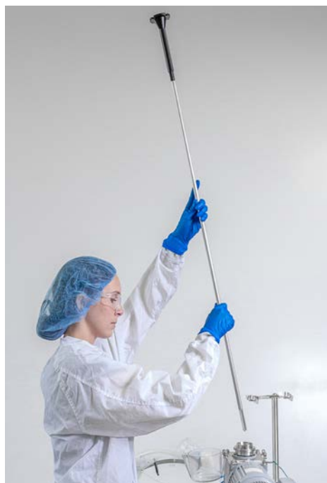
Figure 3.16. Loading drive shaft.
