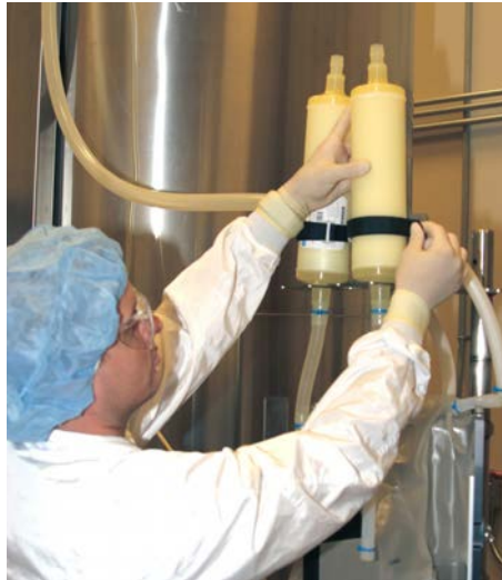
Figure 3.81. Securing vent filters.
