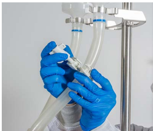
Figure 3.69. Clamping the exhaust lines prior to filling the BPC with air.
