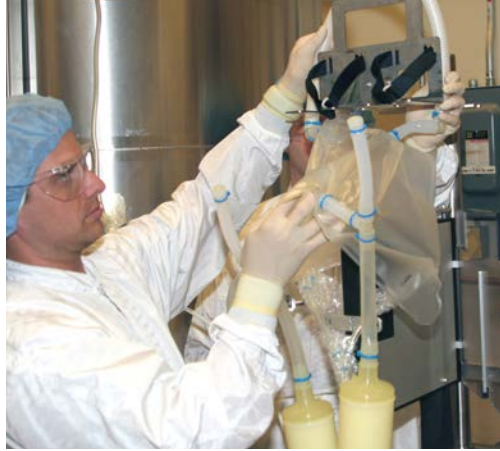
Figure 3.79. Routing gas inlet lines.
