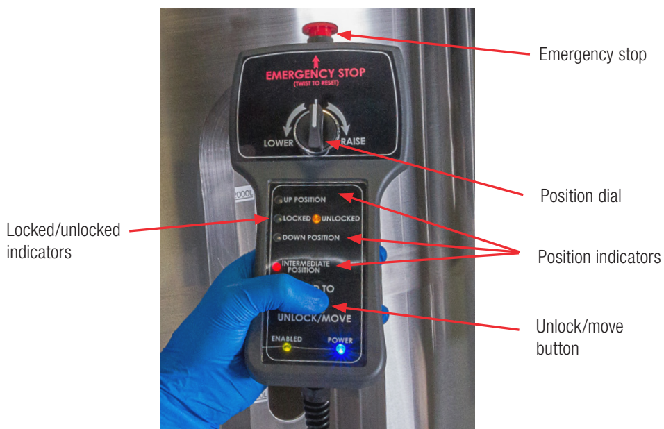
Figure 2.8. Handheld controller for motor lifts.
