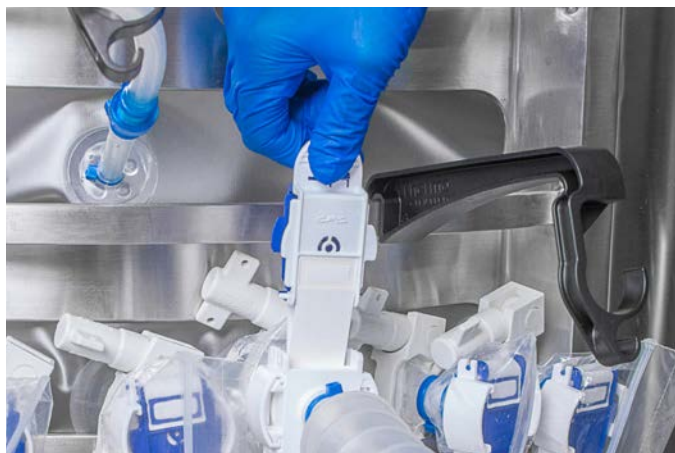
Figure 3.116. Pulling tabs to remove paper membranes.
