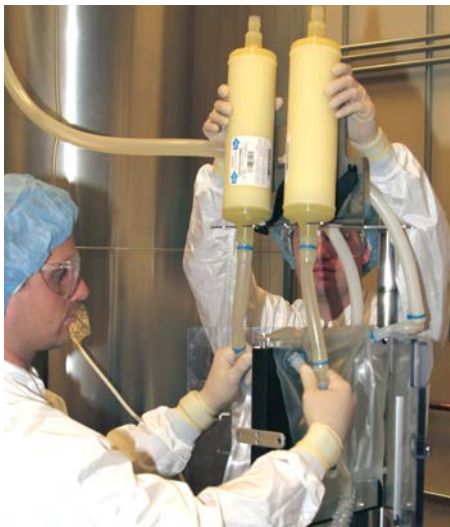
Figure 3.80. Placing vent filters.
