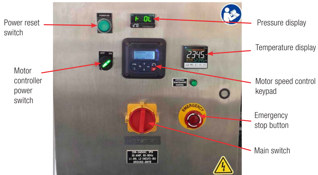
Figure 3.121. Front view of E-Box for 50–2,000 L S.U.B.s.
