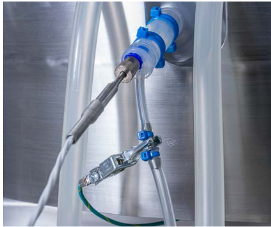
Figure 3.107. Grounding cable connected
