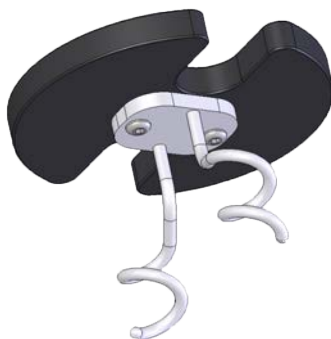
Figure 1.22. Figure 1.22. Sparge line support.
