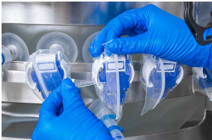
Figure 3.111. Pulling the tear strip.
