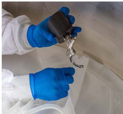
Figure 3.61. Connecting tabs to BPC lift.
