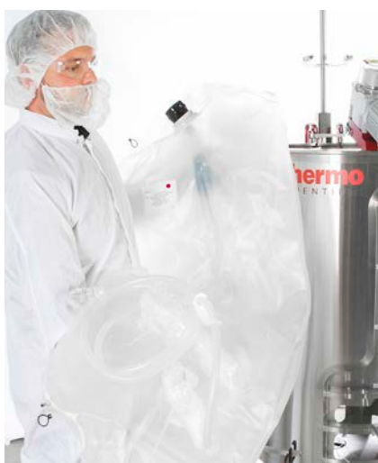
Figure 3.1. BPC removed from protective double polybags.
