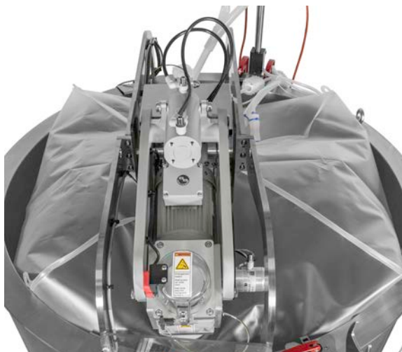
Figure 1.16. Motor lift for 1,000–2,000 L systems.
