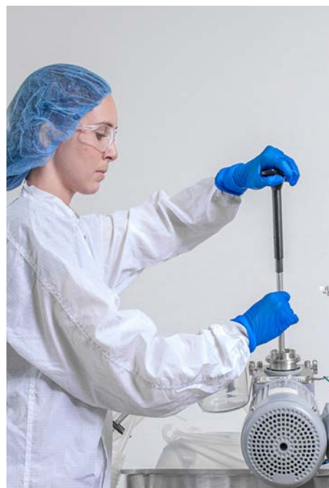
Figure 3.17. Twisting drive shaft to aid insertion.
