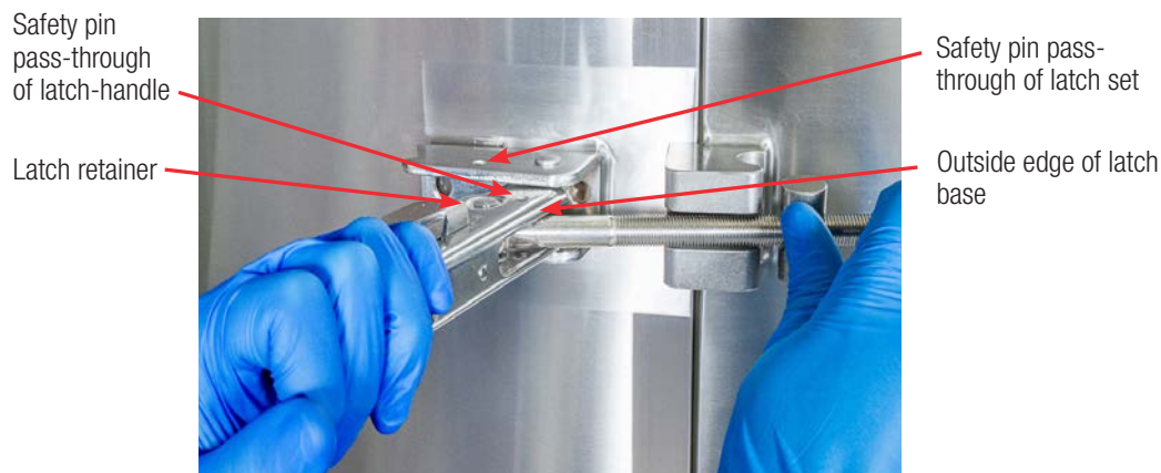
Figure 3.104. Latch access door.
