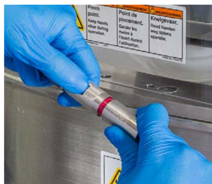
Figure 3.95. Sliding sleeve exposing red "not locked" indicator.
