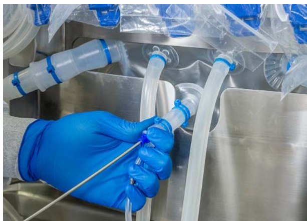
Figure 3.106. Insertion of the RTD into the thermowell.
