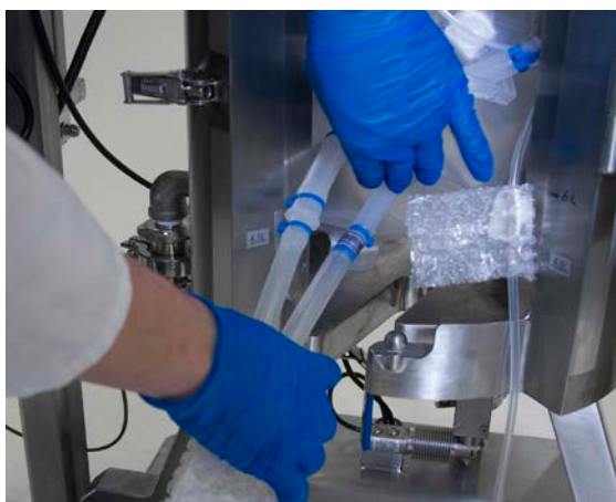
Figure 3.5. Routing the sparge and bottom drain lines.
