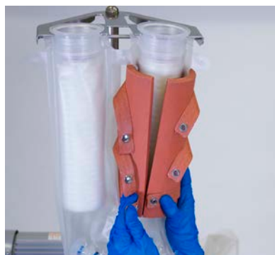
Figure 3.68. Snapping a vent filter heater onto the filter.
