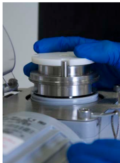
Figure 3.21. Aligning the motor drive keyway.
