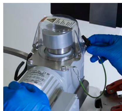
Figure 3.24. Replacing and latching the cover.
