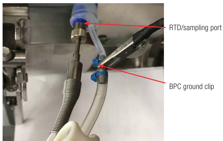
Figure 3.63. Foam sensor ground clip on the RTD.
