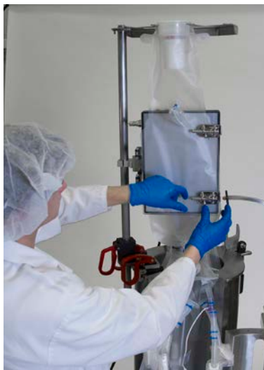
Figure 3.7. Loading of an optional condenser bag.
