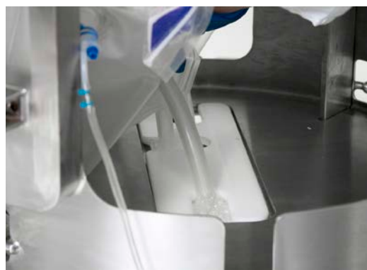
Figure 3.42. Replacing the guide plate.
