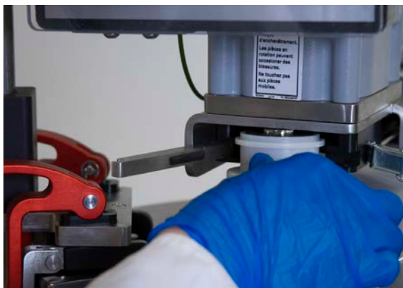
Figure 3.3. Inserting the bearing port.
