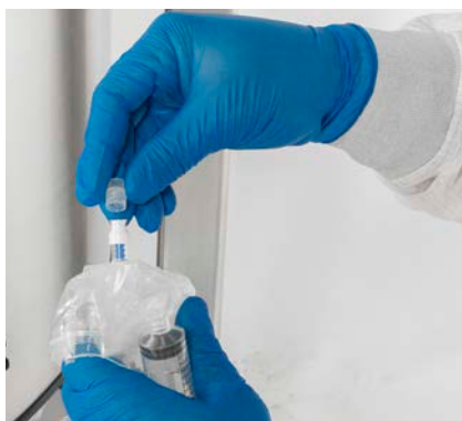
Figure 3.106. Removing the dust cover.
