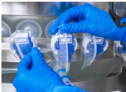
Figure 3.74. Pulling the tear strip.
