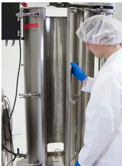
Figure 3.30. Opening the fermentor door.
