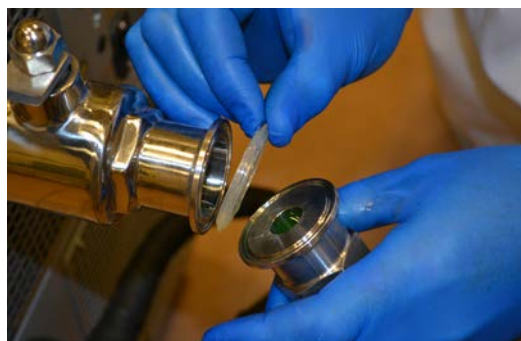
Figure 2.8. Attaching line to a TCU unit.
