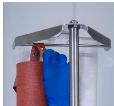
Figure 3.69. Using the snaps to secure the vent filter heater.
