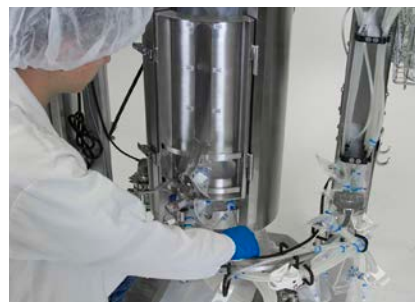
Figure 3.10. Incoming line connection.
