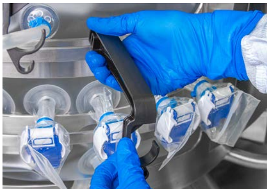
Figure 3.80. Attaching a probe clip.
