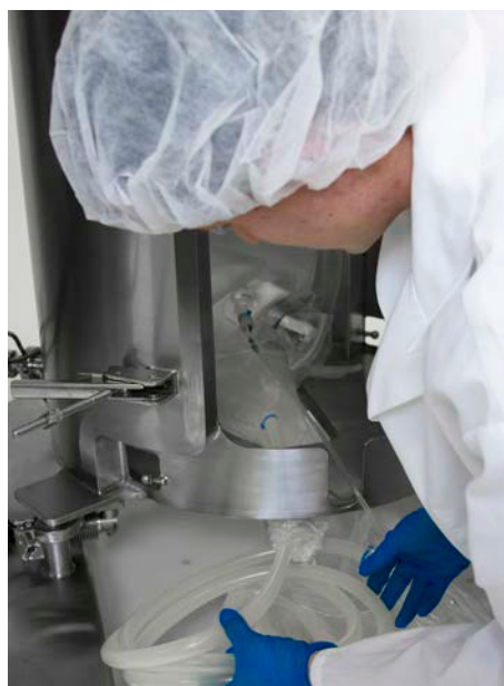
Figure 3.43. Sparge and drain line extension.
