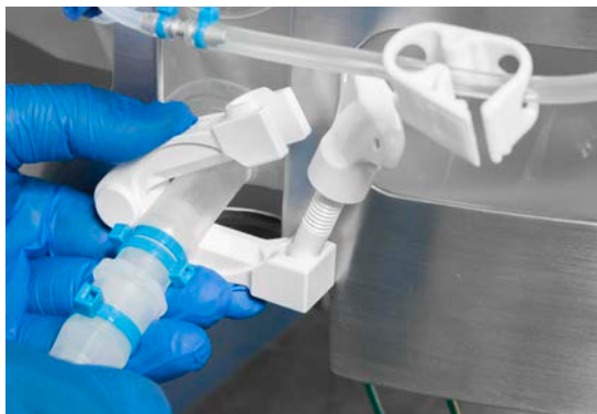
Figure 3.25. Closing bar clamp on drain line.
