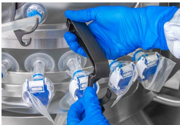
Figure 3.58. Attaching a probe clip.
