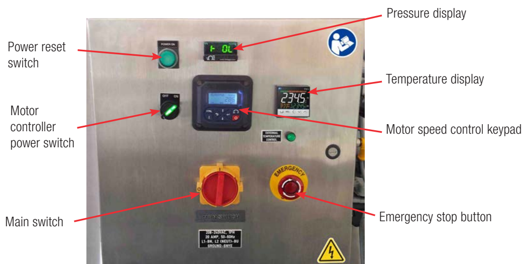
Figure 3.104. Front view of typical S.U.F. E-Box.
