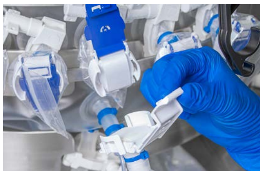
Figure 3.77. Opening the protective cover pull tab on the line set.
