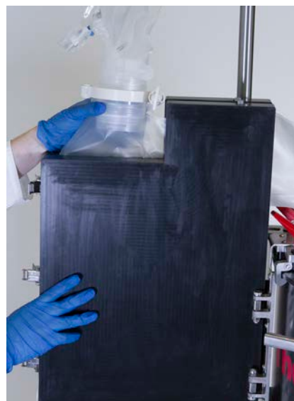
Figure 3.40. Closing the condenser door.
