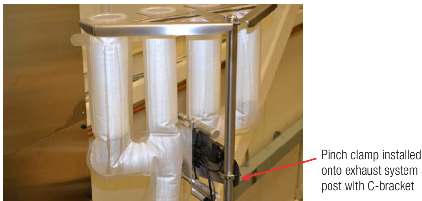
Figure 2.13. Pinch clamp installed on a 300 L S.U.F.
