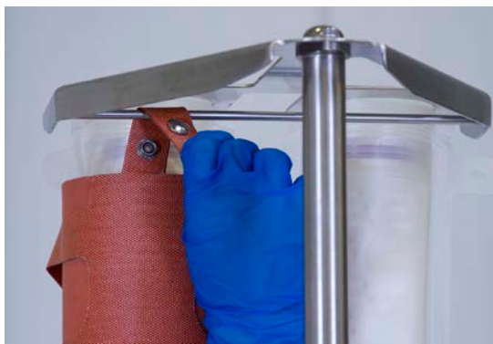
Figure 3.8. Installing an exhaust filter heater.
