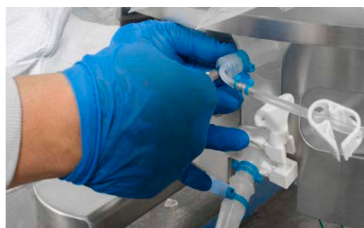
Figure 3.27. Securing the RTD by twisting the luer lock collar.
