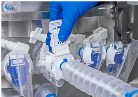
Figure 3.78. Squeezing connectors together.
