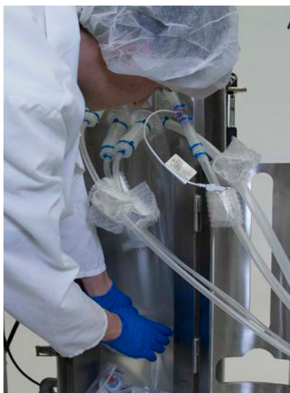
Figure 3.13. Aligning the connector ports and probes.
