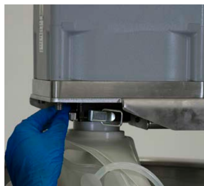
Figure 3.38. Latching the bearing port.
