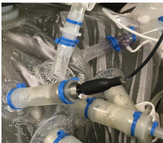
Figure 3.62. Foam sensor wire connected in port.
