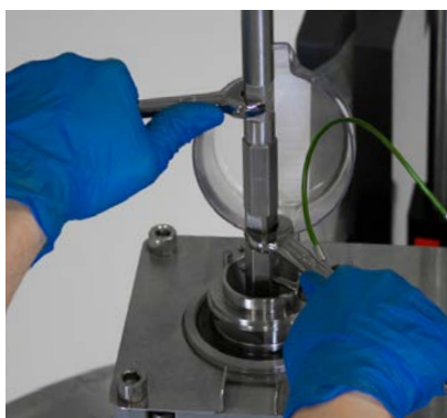
Figure 3.53. Tightening the drive shaft connections.
