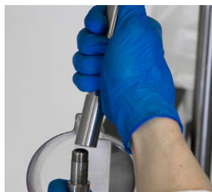
Figure 3.54. Connecting the upper drive shaft segment.
