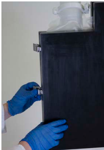
Figure 3.67. Closing and latching the condenser door.
