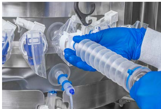
Figure 3.81. Installing the pre-sterilized sensor.
