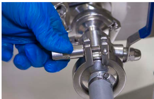
Figure 2.4. Attaching a TCU hose to the water jacket port.
