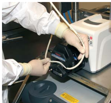
Figure 3.70. Loading pump tubing.
