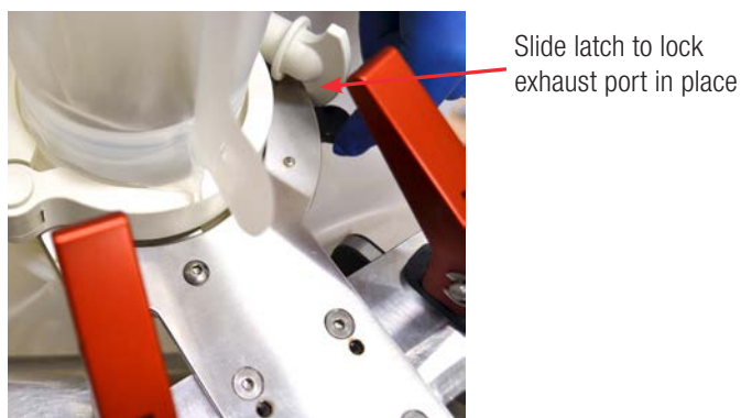
Figure 3.36. Locking the exhaust port.
