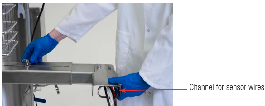
Figure 4.17. Adjustable arm and channel for sensor wires (back view).
