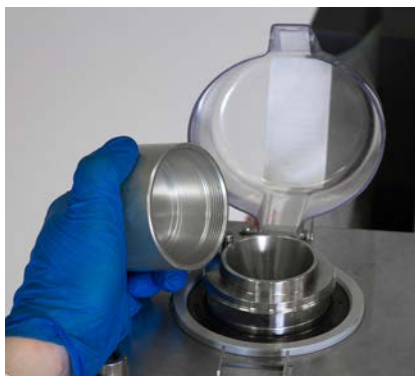
Figure 3.50. Removing the drive shaft cap.
