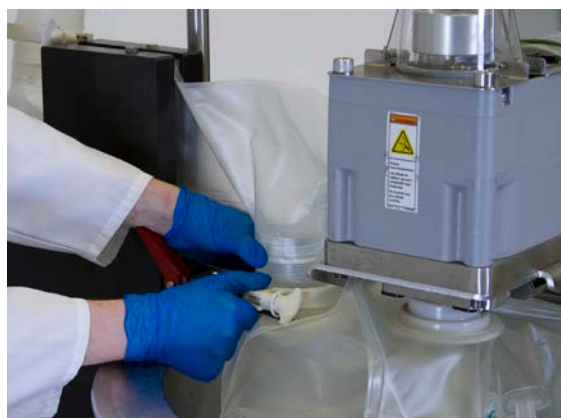
Figure 3.34. Inserting the condenser into the exhaust port in a holder at the top of the tank.
