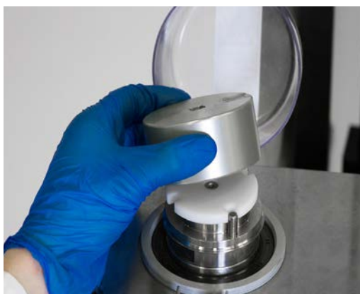
Figure 3.56. Replacing the drive shaft cap.
