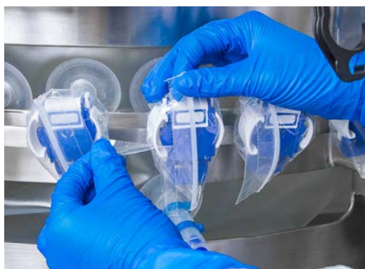
Figure 3.74. Pulling the tear strip.
