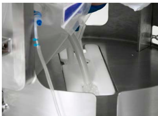
Figure 3.42. Replacing the guide plate.
