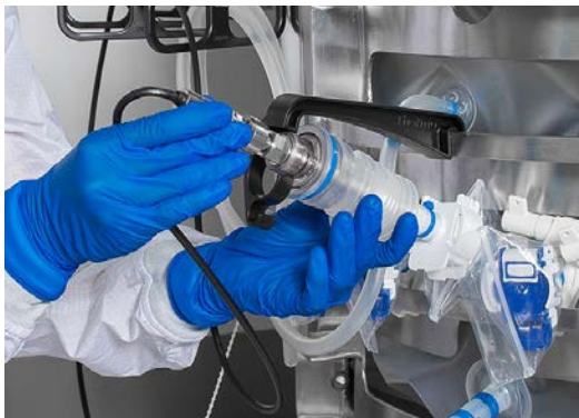
Figure 3.83. Lifting the probe upward into the spring.
