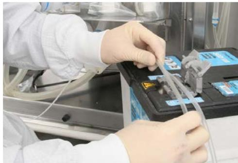
Figure 3.108. Tubing welder.
