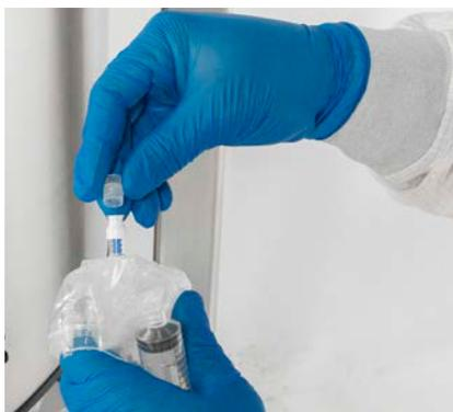
**Figure 3.106. Removing the dust cover.**
