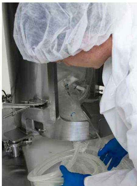
Figure 3.43. Sparge and drain line extension.
