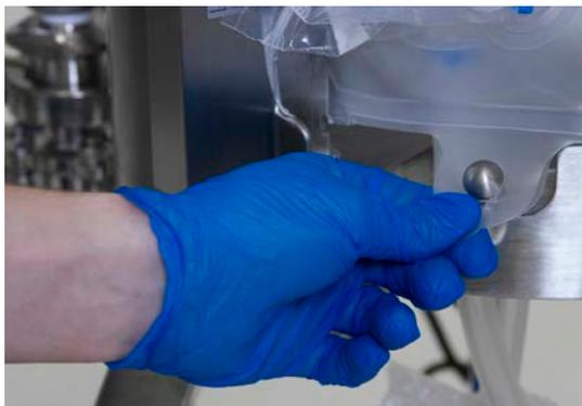
Figure 3.12. Aligning a hanging tab with the pin.
