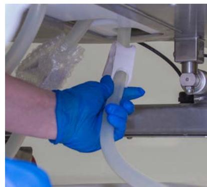
Figure 3.60. Placing a clamp on the drain line.
