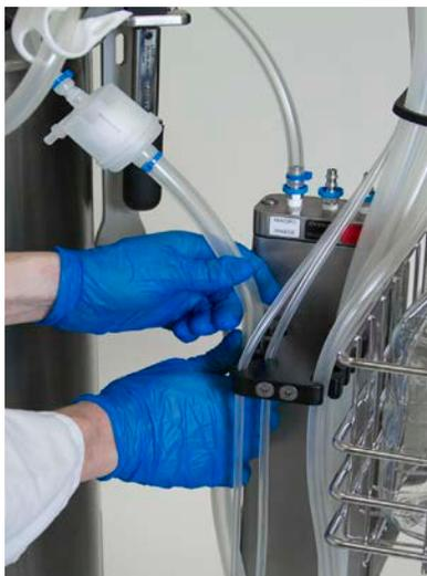
Figure 3.9. Line setup on the cable management system.
