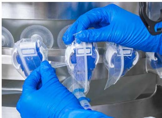
Figure 3.74. Pulling the tear strip.
