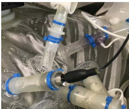
Figure 3.28. Foam sensor wire plugged in.
