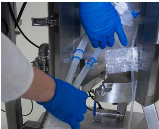
Figure 3.5. Routing the sparge and bottom drain lines.
