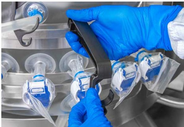
Figure 3.58. Attaching a probe clip.
