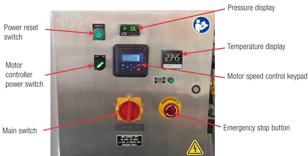
Figure 3.104. Front view of typical S.U.F. E-Box.
