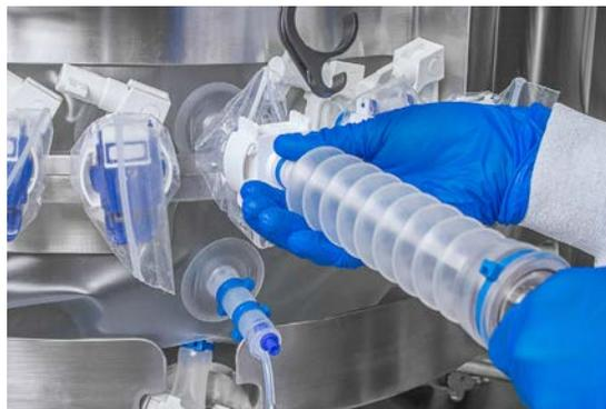
Figure 3.81. Installing the pre-sterilized sensor.
