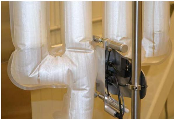
Figure 3.44. Pinch clamp installed on a 300 L BPC.
