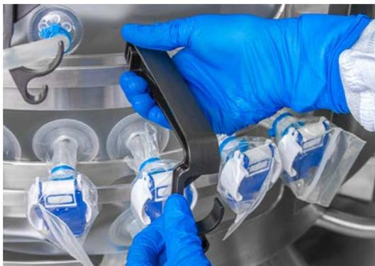
Figure 3.80. Attaching a probe clip.
