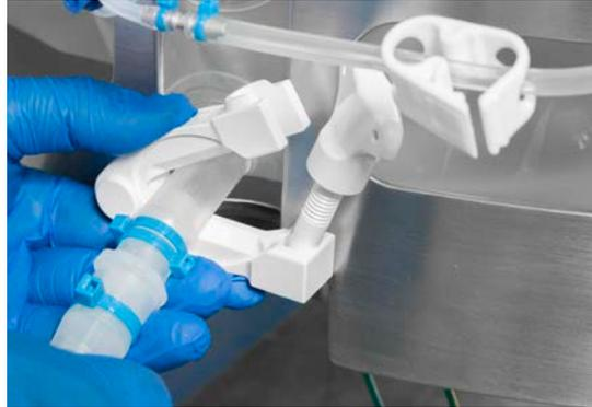
Figure 3.25. Closing bar clamp on drain line.
