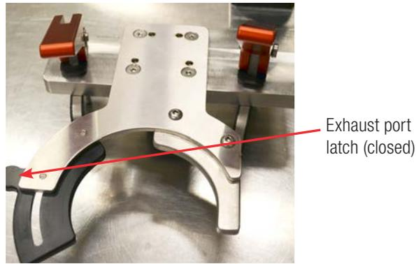
Figure 3.35. Exhaust port sliding latch (removed from the tank).
