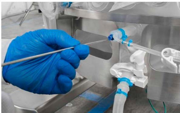
Figure 3.61. Inserting a sensor into the thermowell.
