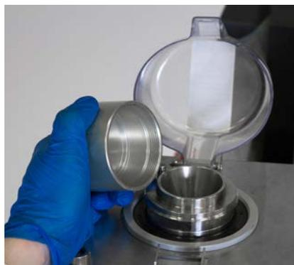
Figure 3.50. Removing the drive shaft cap.
