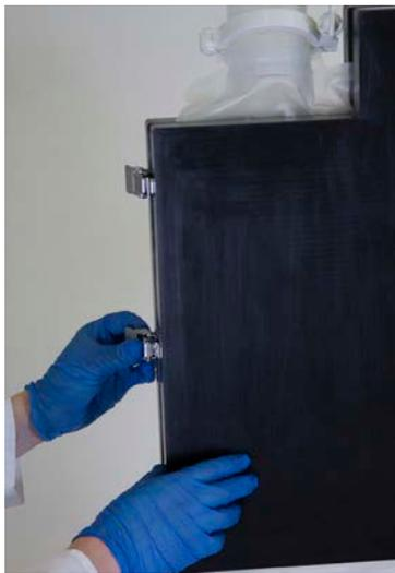
**Figure 3.67. Closing and latching the condenser door.**
