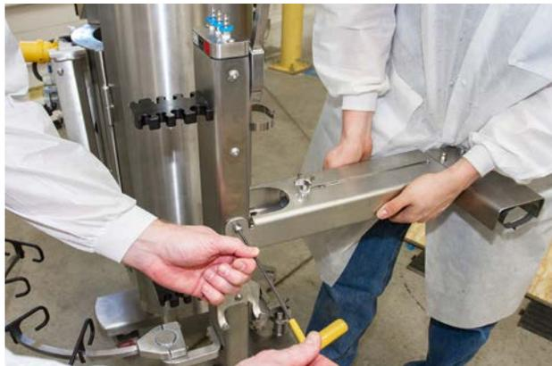
Figure 2.14. Attaching arm to cable management system.
