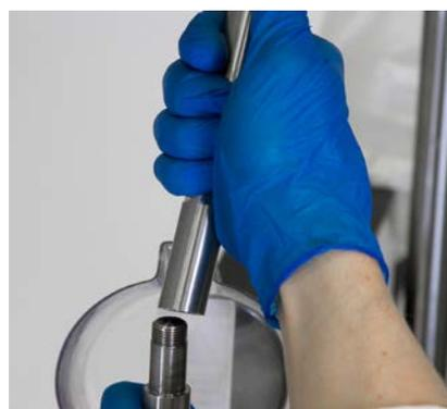
Figure 3.54. Connecting the upper drive shaft segment.
