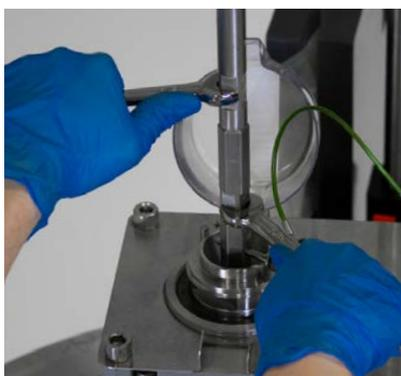
Figure 3.53. Tightening the drive shaft connections.
