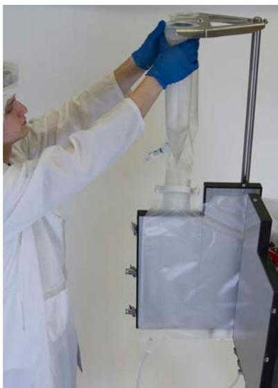
Figure 3.39. Exhaust filter and condenser setup.
