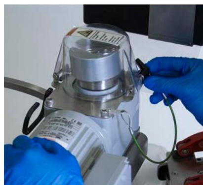
Figure 3.24. Replacing and latching the cover.
