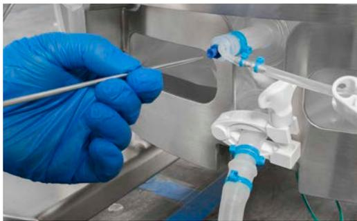
Figure 3.26. Inserting the RTD into the thermowell.
