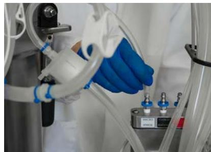
Figure 3.11. Incoming line connection to a direct sparger filter.
