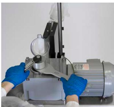
Figure 3.23. Tightening the cap.
