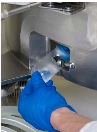
Figure 3.46. Attaching hanging tabs.
