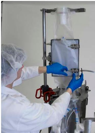
Figure 3.7. Loading of an optional condenser bag.
