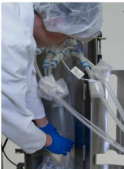
Figure 3.13. Aligning the connector ports and probes.
