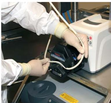
Figure 3.70. Loading pump tubing.
