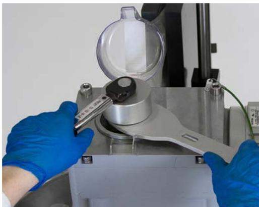
Figure 3.57. Tightening the cap with wrenches.
