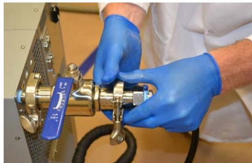
Figure 2.9. Attaching a clamp to a line.
