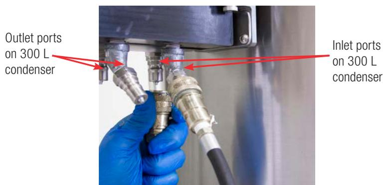
**Figure 2.11.** Attaching TCU lines to a condenser on a 300 L S.U.F. unit.
