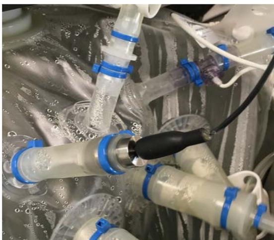
Figure 3.62. Foam sensor wire connected in port.
