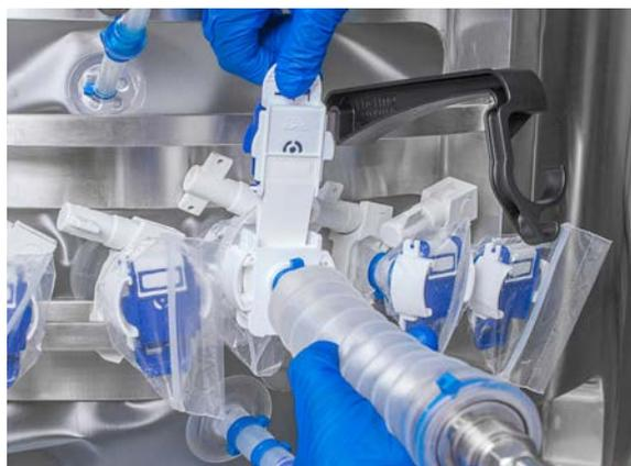
Figure 3.79. Pulling tabs to remove the paper membranes.
