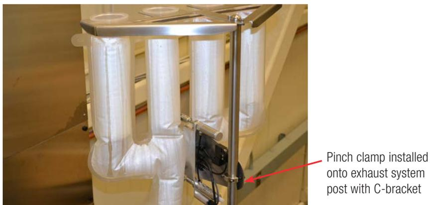
Figure 2.13. Pinch clamp installed on a 300 L S.U.F.
