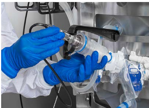
Figure 3.83. Lifting the probe upward into the spring.
