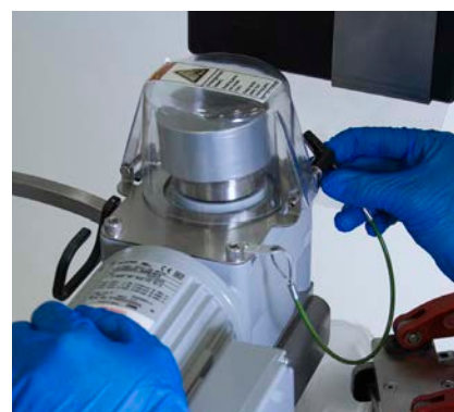
Figure 3.24. Replacing and latching the cover.
