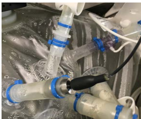
Figure 3.28. Foam sensor wire plugged in.
