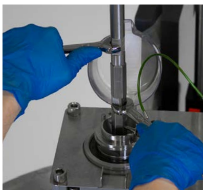
Figure 3.53. Tightening the drive shaft connections.
