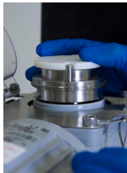
Figure 3.21. Aligning the motor drive keyway.
