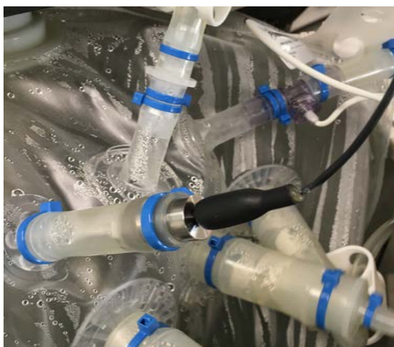
Figure 3.62. Foam sensor wire connected in port.
