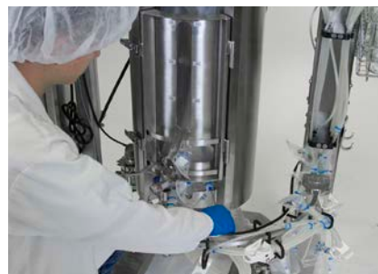
Figure 3.10. Incoming line connection.
