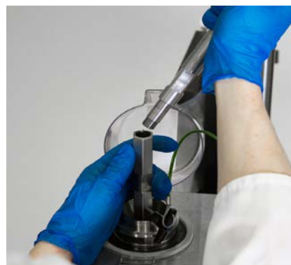
Figure 3.52. Connecting the middle section of the drive shaft.
