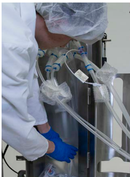
Figure 3.13. Aligning the connector ports and probes.
