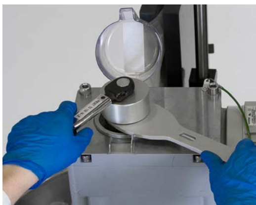
Figure 3.57. Tightening the cap with wrenches.
