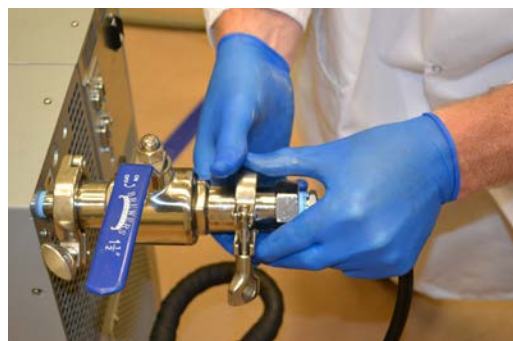
Figure 2.9. Attaching a clamp to a line.
