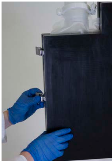
Figure 3.67. Closing and latching the condenser door.
