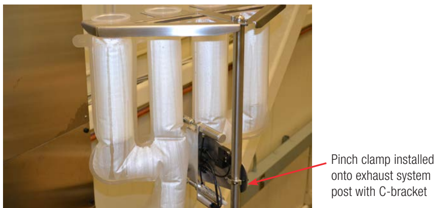
Figure 2.13. Pinch clamp installed on a 300 L S.U.F.
