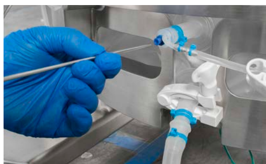
Figure 3.26. Inserting the RTD into the thermowell.
