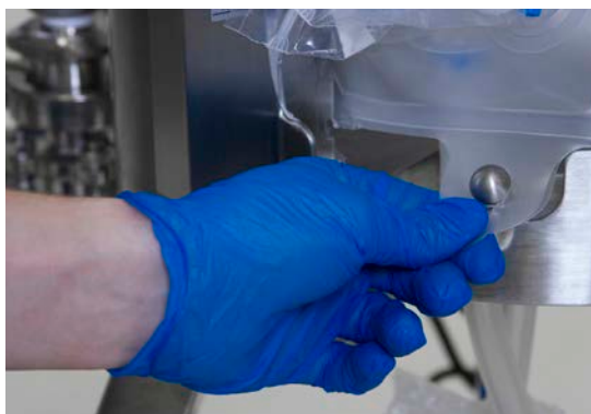
Figure 3.12. Aligning a hanging tab with the pin.
