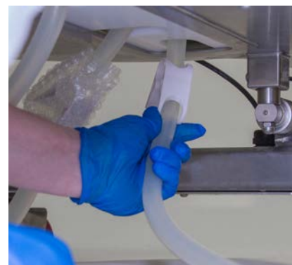
Figure 3.60. Placing a clamp on the drain line.
