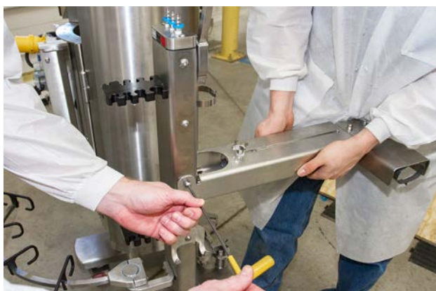
Figure 2.14. Attaching arm to cable management system.
