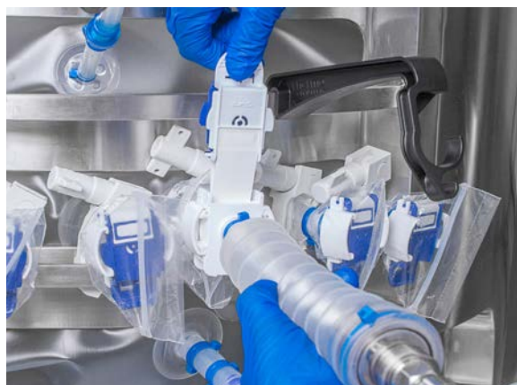
Figure 3.79. Pulling tabs to remove the paper membranes.
