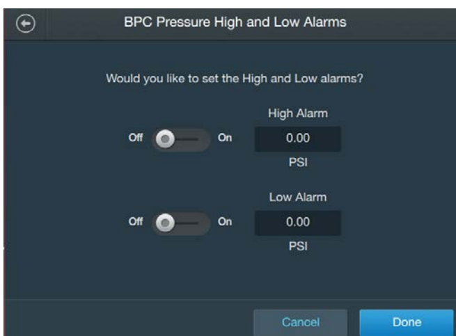
Figure 3.26. BPC Pressure High and Low Alarms screen.
