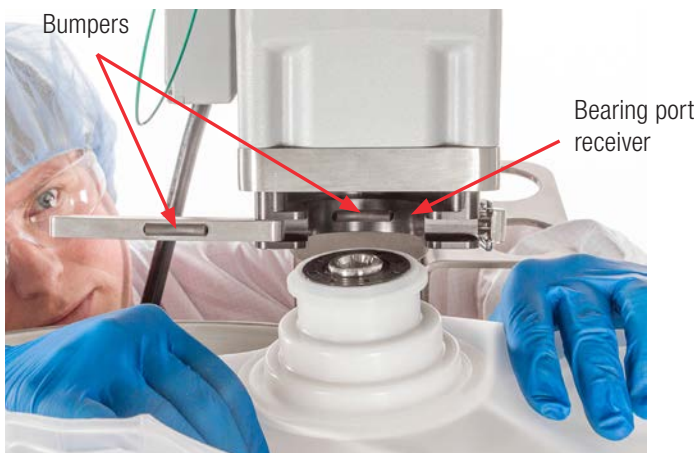
Figure 5.6. Inserting the bearing port into the receiver.
