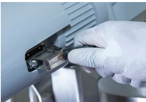
Figure 3.7. Motor control connection.
