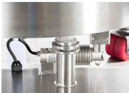
Figure 8.20. Mettler Toledo MTB load cell for 50–1,000 L S.U.M. units.
