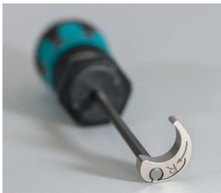
Figure 3.8. Supplied tool for connecting communication cables.
