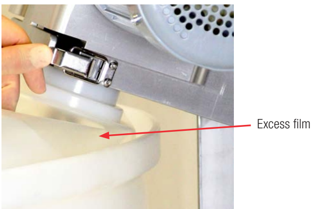
Figure 5.9. Properly loaded BPC.
