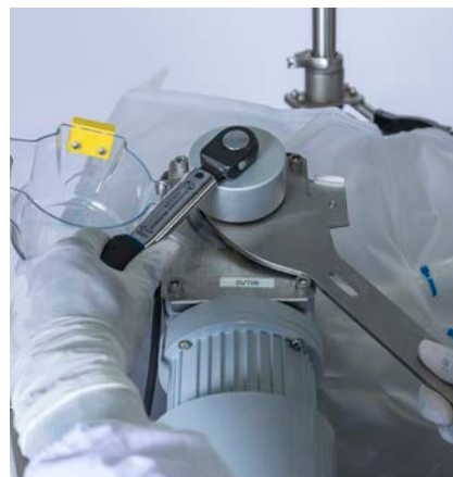
Figure 5.21. Tightening the cap.
