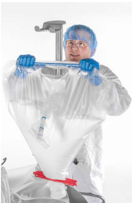
Figure 6.3. Hanging the Powdertainer on the support arm.
