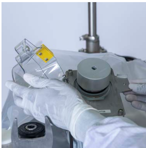
Figure 5.16. Removing the safety cover.
