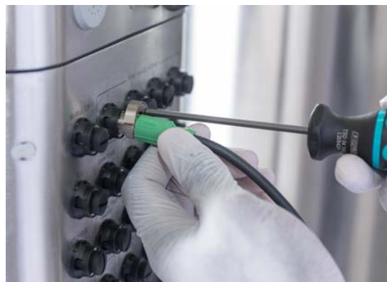
Figure 3.9. Connecting communication cables to the Touchscreen Console.
