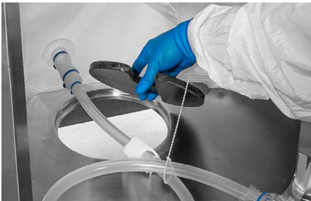
Figure 5.4. Routing the drain line through the tank.
