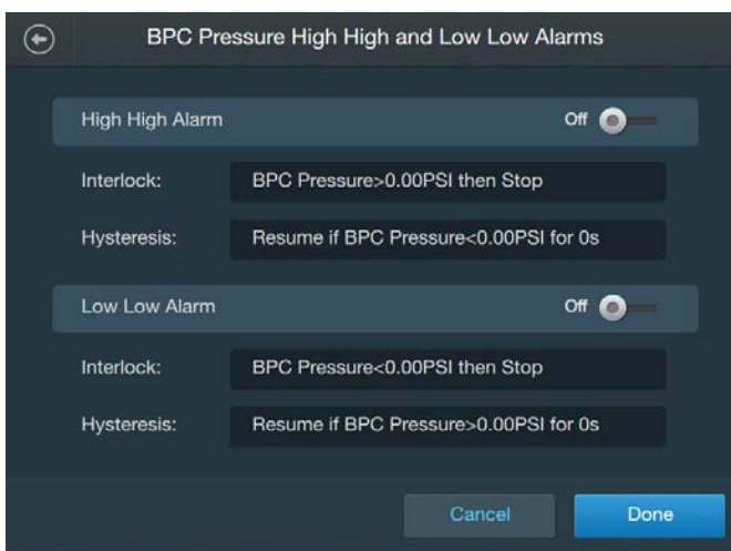
Figure 3.27. BPC Pressure High High and Low Low Alarms screen.
