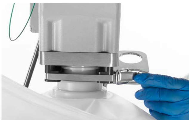
Figure 5.7. Closing and latching the bearing hub receiver.
