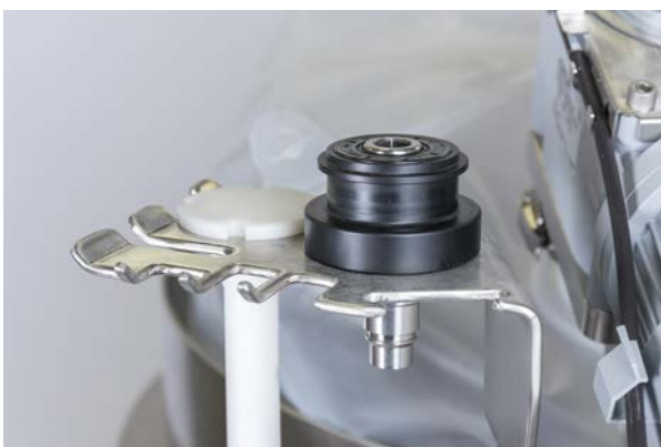
Figure 2.6. Drive shaft and bearing hub stored in bracket.
