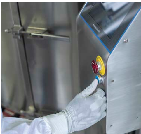
Figure 3.10. Pressing the blue power-on restart button.
