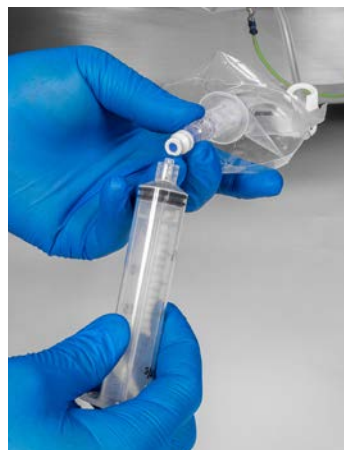
Figure 6.10. Inserting sampling syringe.
