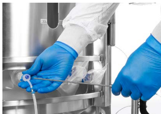
Figure 5.43. Inserting temperature sensor.
