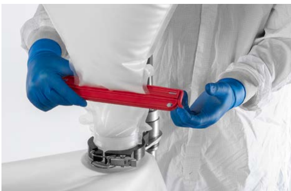
Figure 6.7. Releasing the Powdertainer feed clamp.
