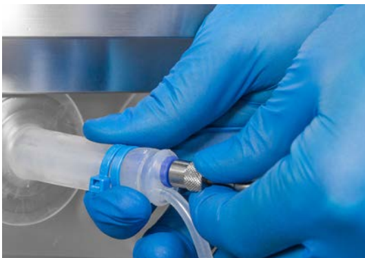
Figure 5.44. Twisting the temperature sensor to seat it properly.
