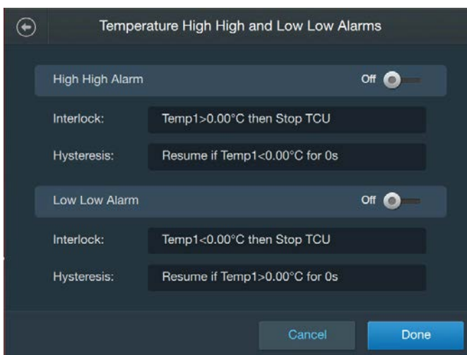
Figure 3.42. High High and Low Low Alarms screen.
