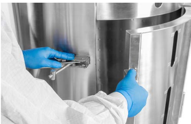
Figure 5.1. Opening the door on a 500 L S.U.M.
