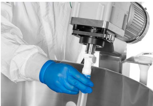
Figure 5.26. Attaching the impeller sleeve.
