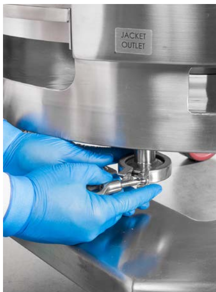
Figure 2.7. Removing tri-clamp on water jacket outlet.
