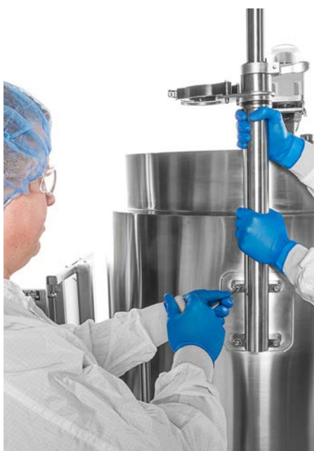
Figure 2.9. Installing Powdertainer arm.
