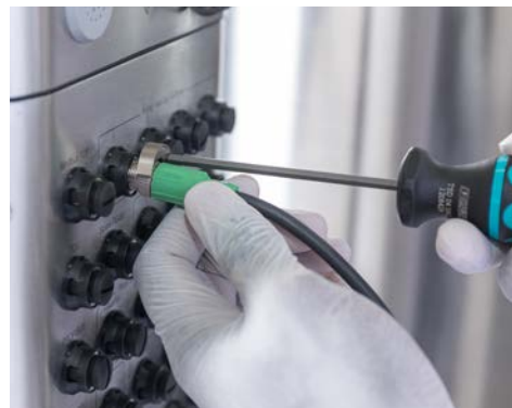
Figure 3.3. Connecting pumps to the Touchscreen Console.
