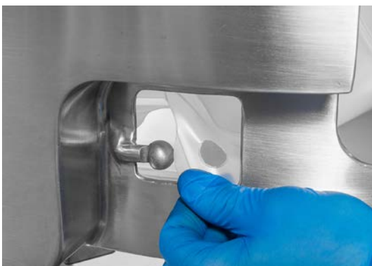
Figure 5.8. Aligning BPC positioning tabs with pins.
