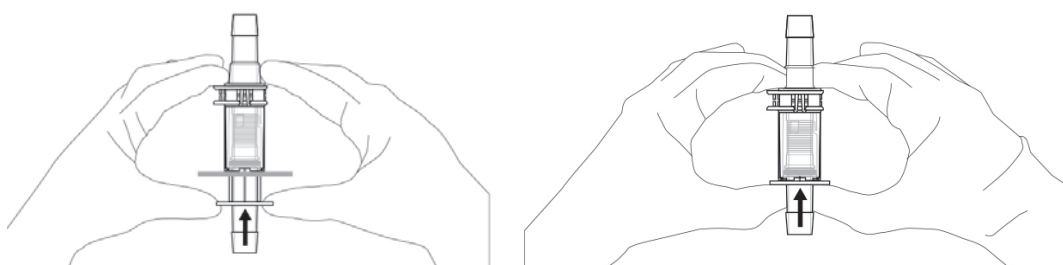
Figure 5.41. Pushing the thumb rest toward the barrel.
