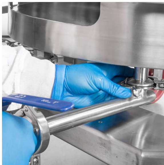
Figure 2.8. Attaching fitting to water jacket port.
