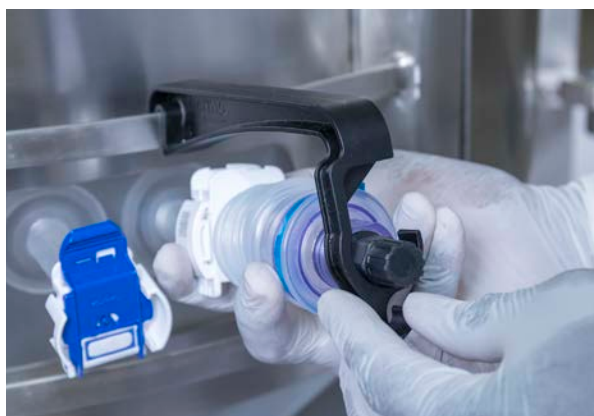
Figure 5.48. Placing collapsed probe assembly into the probe clip.
