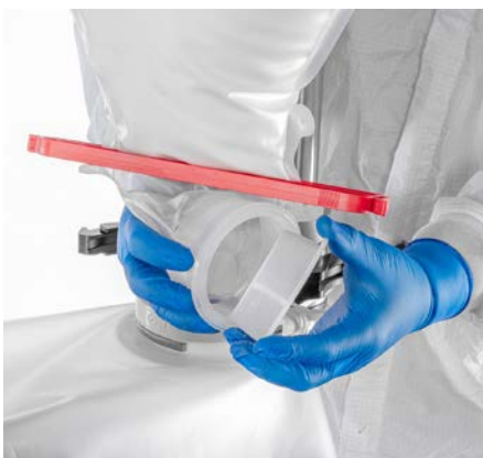
Figure 6.4. Removing the cap from the Powdertainer.
