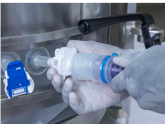
Figure 5.47. Compressing the probe bellows.
