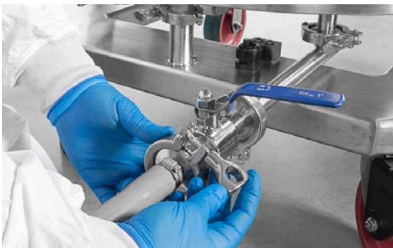
Figure 2.11. Connecting the TCU to the water jacket.
