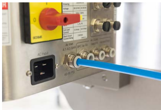
Figure 3.4. Air line connected to the back of the Touchscreen Console.
