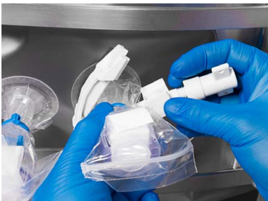
Figure 5.46. Placing tubing clamps.
