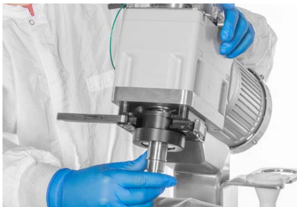
Figure 5.25. Inserting the reusable bearing hub.
