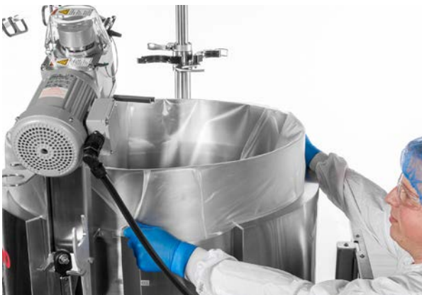
Figure 5.24. Installing the liner.
