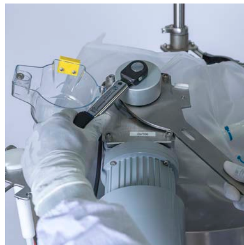
Figure 5.17. Using wrenches to remove cap.
