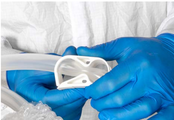
Figure 5.3. Closing line set clamp.
