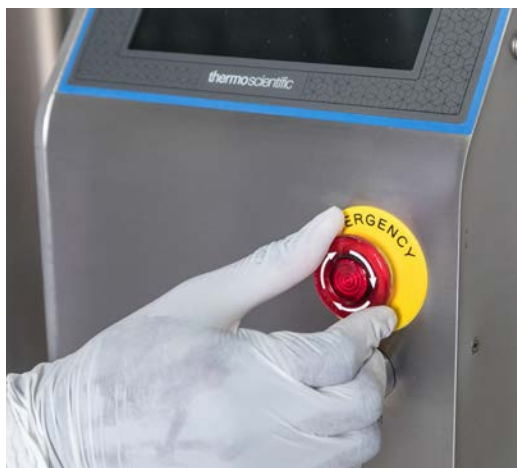
Figure 3.6. Turning knob on the E-Stop clockwise to disengage.
