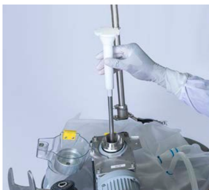
Figure 5.18. Inserting drive shaft.
