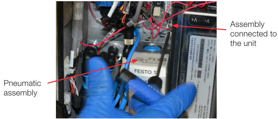
Figure 5.27. Using an Allen wrench to disconnect from the unit
