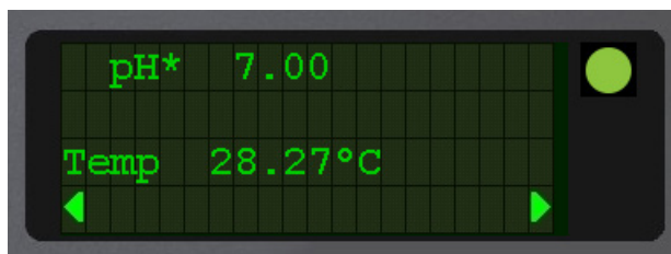
Figure C.9. Asterisk next to parameter name, indicating non-factory calibration in use.
