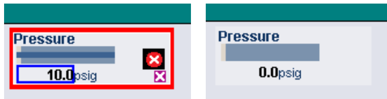
Figure 3.30. Pressure shown before (left) and after (right) taring on the Pressure control module.
