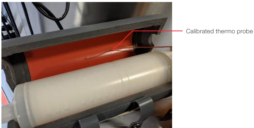
Figure 3.27. Thermo probe placed in the vent filter heater.
