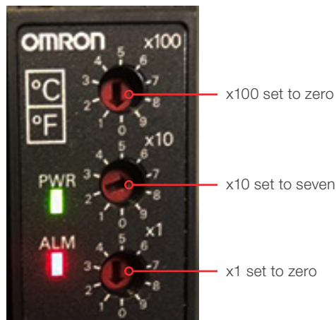
Figure 3.42. Rotary switches set to 70°C.
